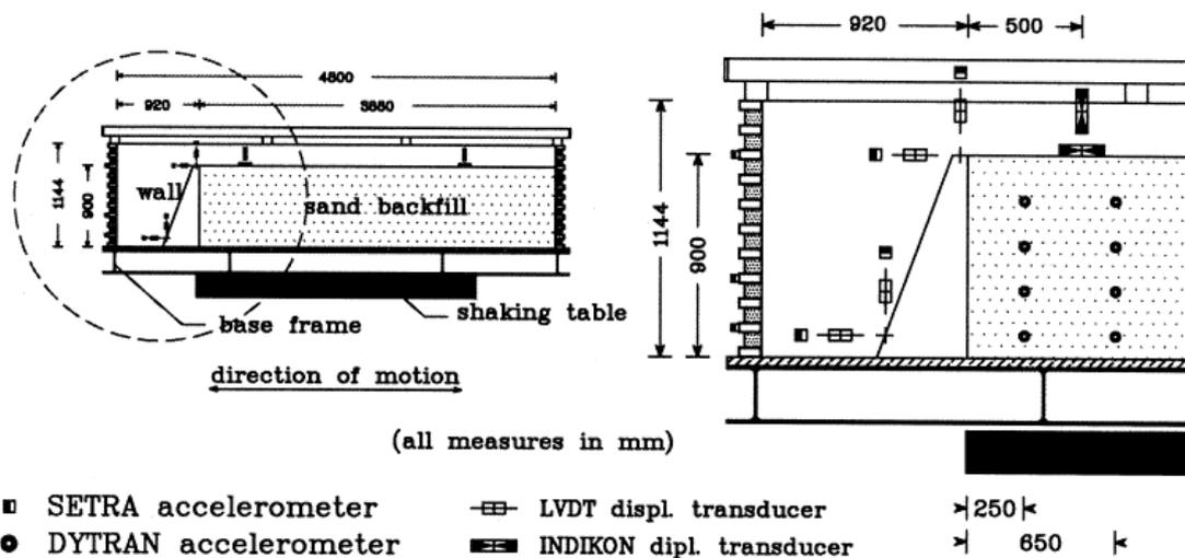
Figure 2: Elevation of the shear stack showing the location of the retaining wall and the associated instrumentation
