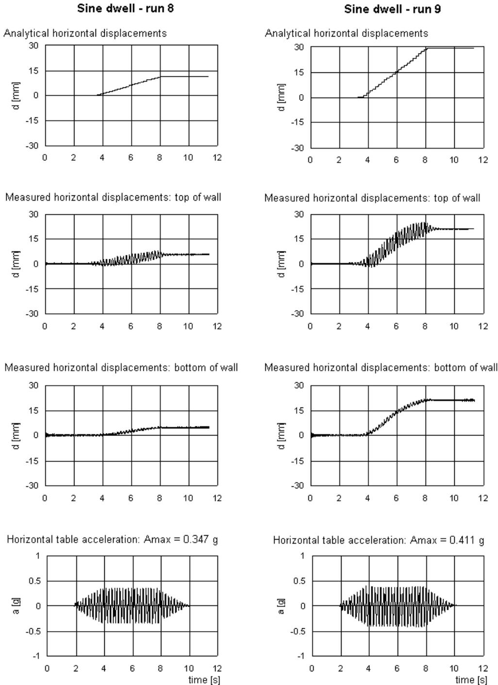
**Figure 4: Comparison between the responses generated by the analytical model and the experimental tests**
