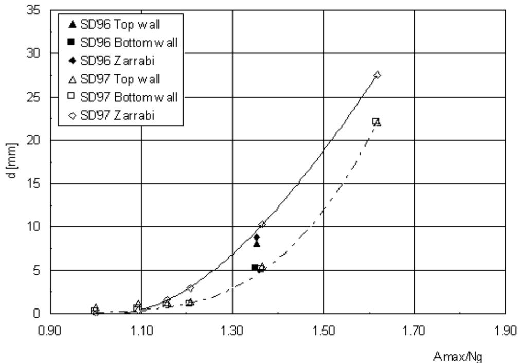
Figure 5: Comparison between measured and Zarrabi computed displacements
