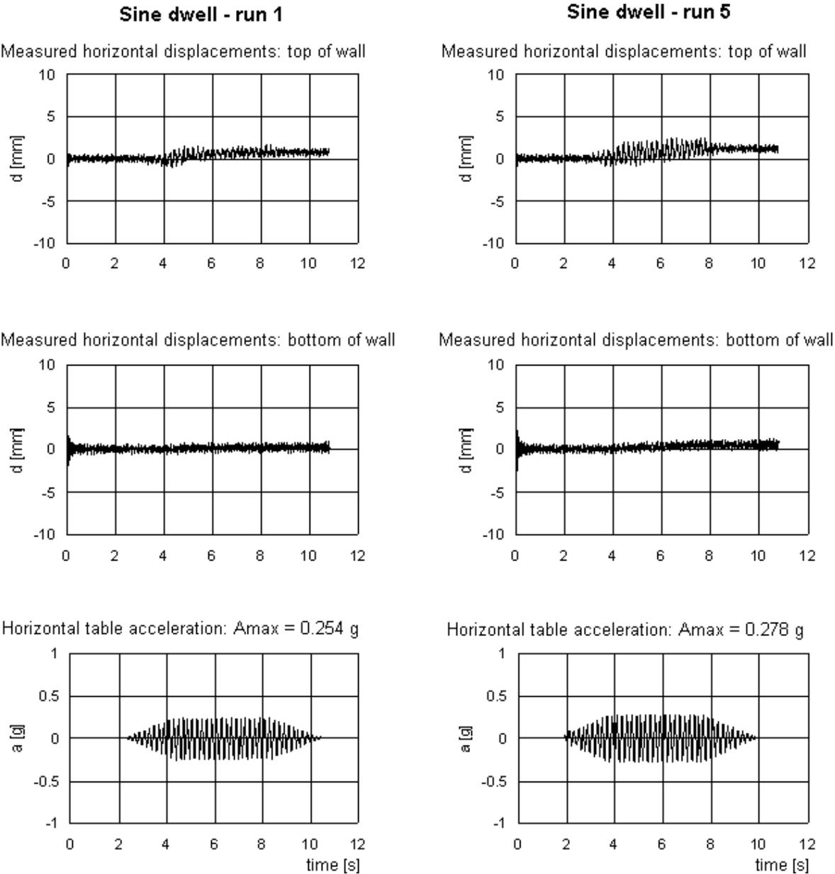
**Figure 3: Displacements for table accelerations close to the limit acceleration of the wall-soil system**
