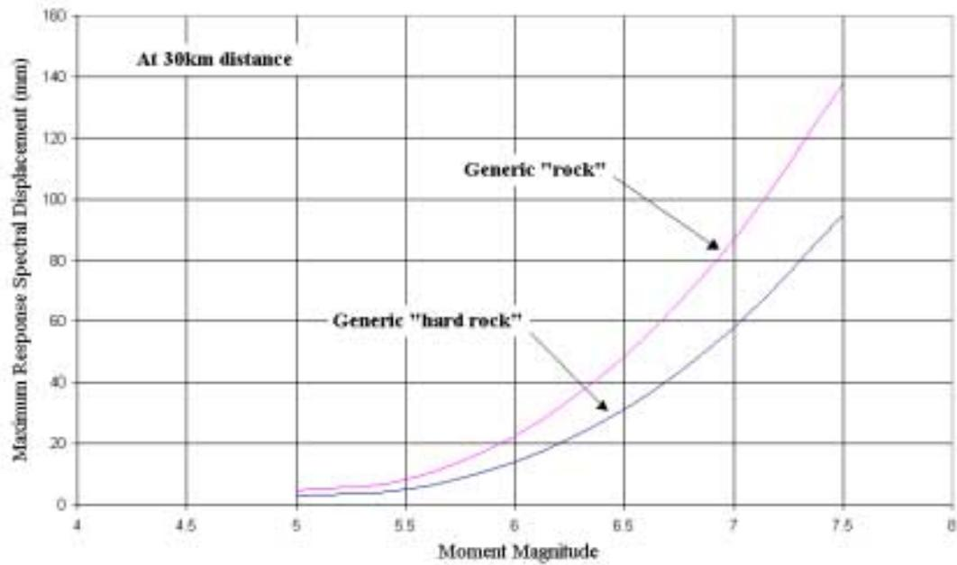
Figure 2 Correlations of Maximum Response Spectral Displacement with Moment Magnitude
