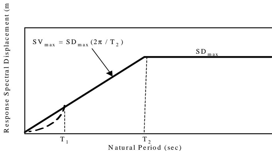
Figure 1 The Bi-linear Displacement Response Spectrum
