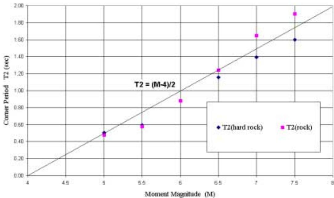
Figure 3 Corner Period of Displacement Response Spectrum
