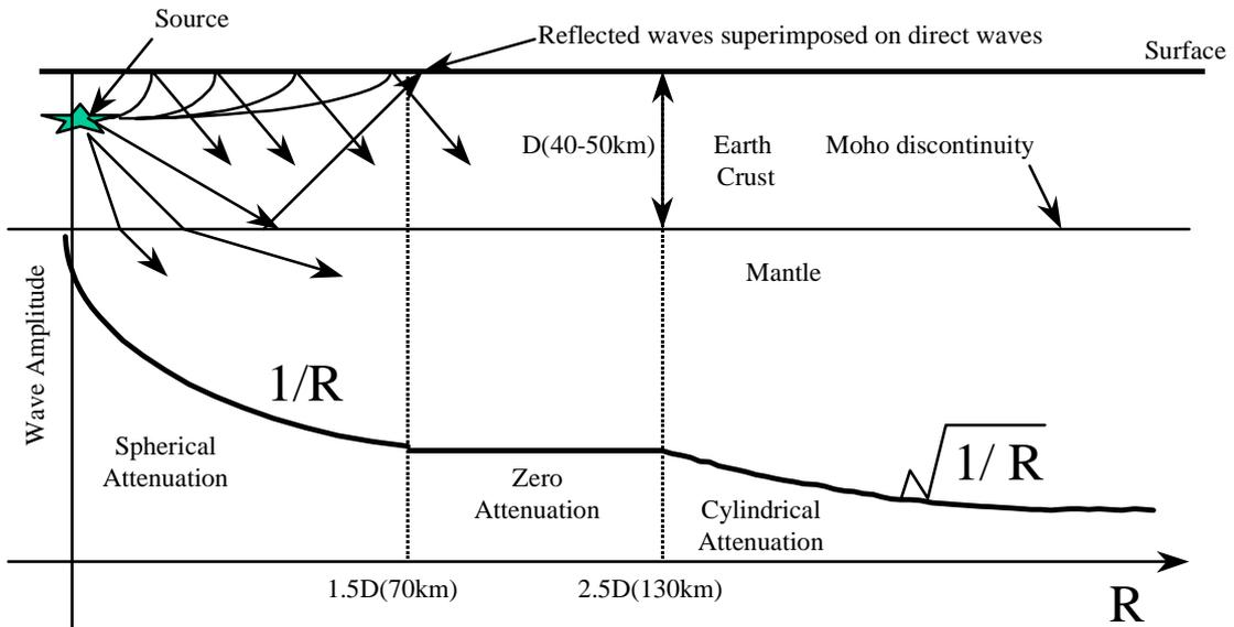
Figure 4 Geometrical Attenuation of Seismic Shear Waves
