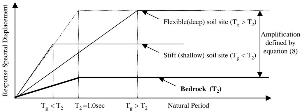
Figure 6 Unified Displacement Response Spectrum Model for Rock and Soil Sites
