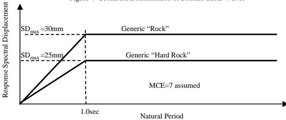
Figure 5 Characteristic Displacement Response Spectra for Generic Rock Sites
