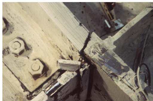
Figure 4: Column failure of specimen PN1
