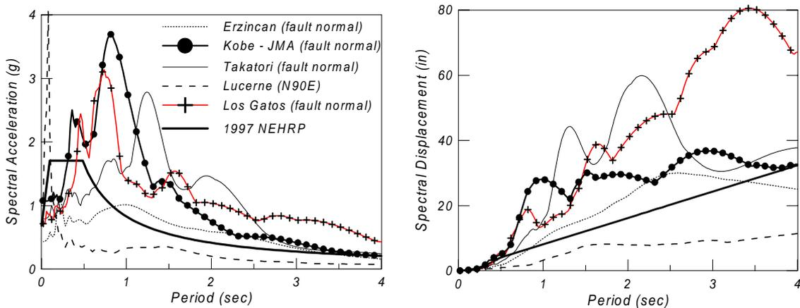
**Figure 2 Comparison of elastic response spectra of ground motions studied with the design spectra according to the 1997 NEHRP provisions.**
