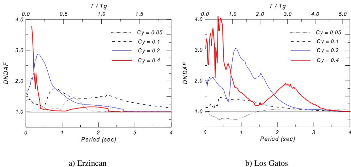
**Figure 6: Degrading-to-nondegrading displacement amplification factors (DNDAF) for systems with high degradation subjected to the Erzincan and Los Gatos records.**
