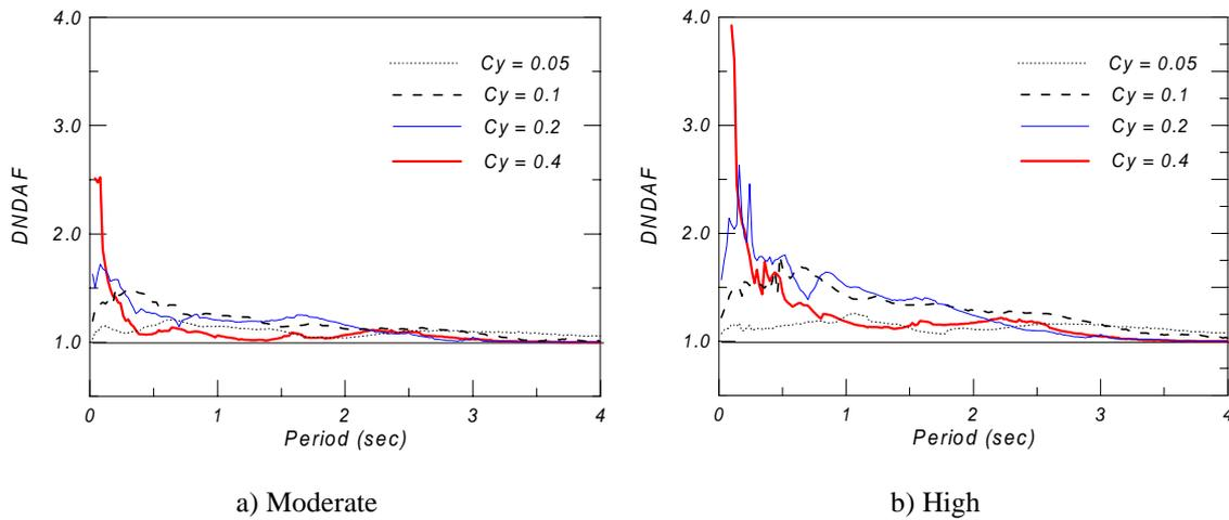
**Figure 7: Average degrading-to-nondegrading displacement amplification factors (DNDAF) for systems with moderate and high degradation characteristics.**
