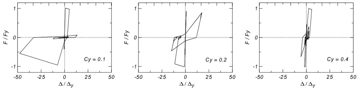
**Figure 5: Hysteretic response for an oscillator of moderate decay characteristics and different strength coefficients subjected to the Los Gatos record ( $T = 1$  second).**
