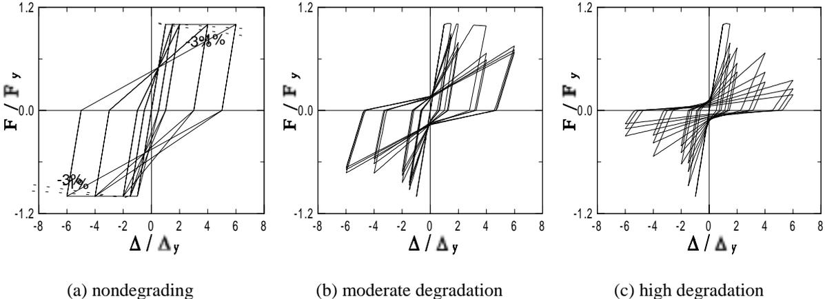
**Figure 1: Hysteretic response characteristics of the degrading systems studied.**
