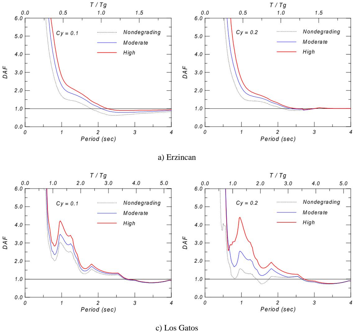
**Figure 4: Displacement amplification factors: a) Erzincan and b) Los Gatos.**
