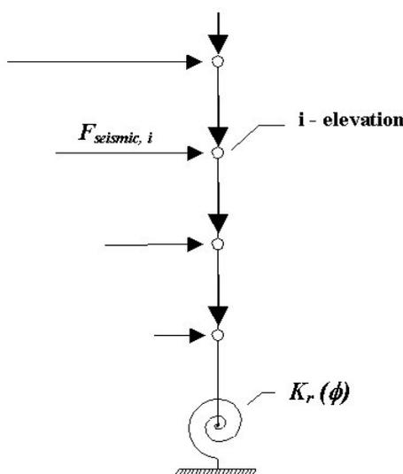
**Fig. 2 – Simplified soil-structure schematization**
