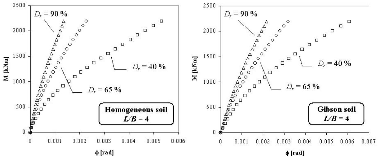
Fig. 3 – Moment-rotation diagrams developed by means of the SOFIA code for  $L/B = 4$
