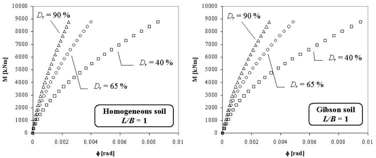
Fig. 4 – Moment-rotation diagrams developed by means of the SOFIA code for  $L/B = 1$
