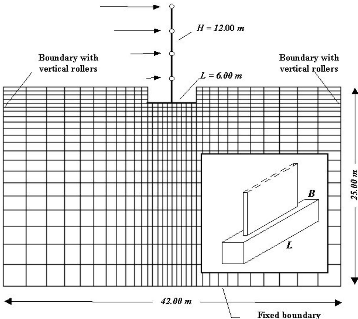
Fig. 1 – Soil-structure system
