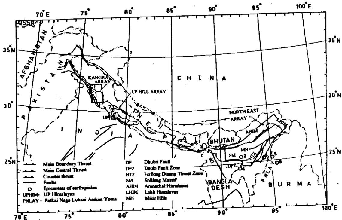
Fig. 1. Strong motion arrays in India deployed by Department of Earthquake Engineering, University of Roorkee. The location of the contributing earthquakes are also shown (o).
