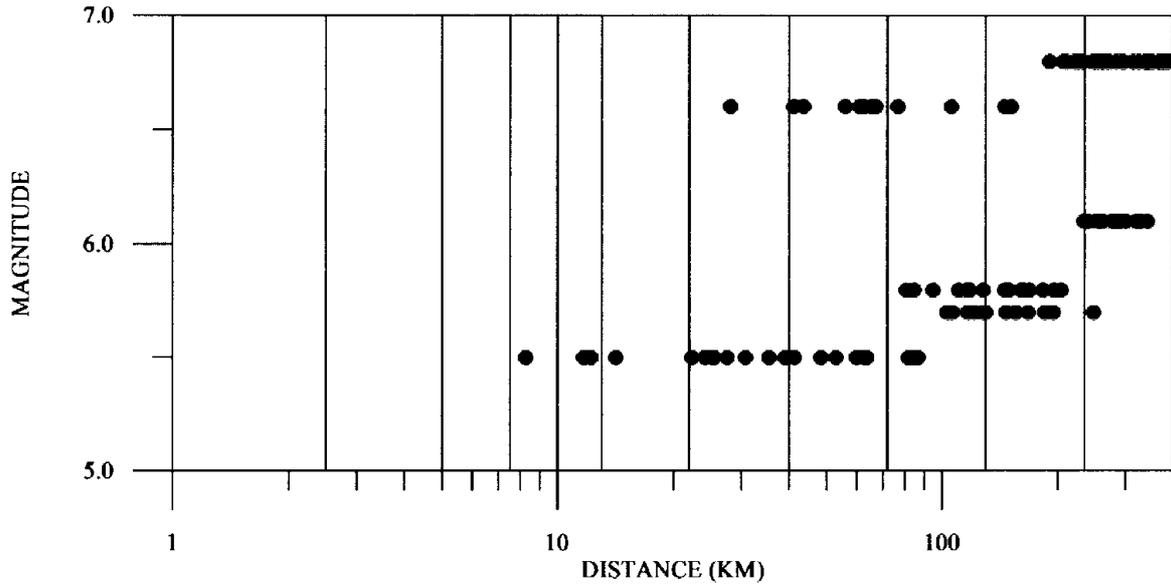
FIG. 2 Magnitude-distance distribution of peak ground vertical acceleration data. The vertical lines drawn are the distance bins used for the weighted non-linear analysis.
