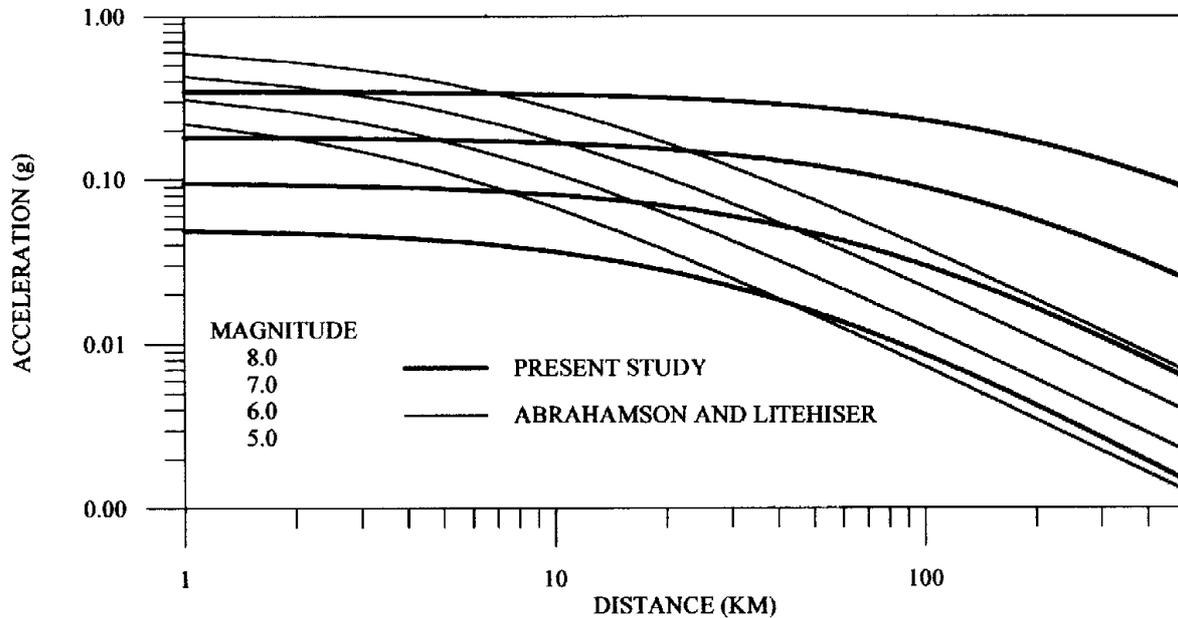
FIG. 4. Comparison of the newly developed attenuation relationship with the relationship given by Abrahamson and Litehiser (1989)
