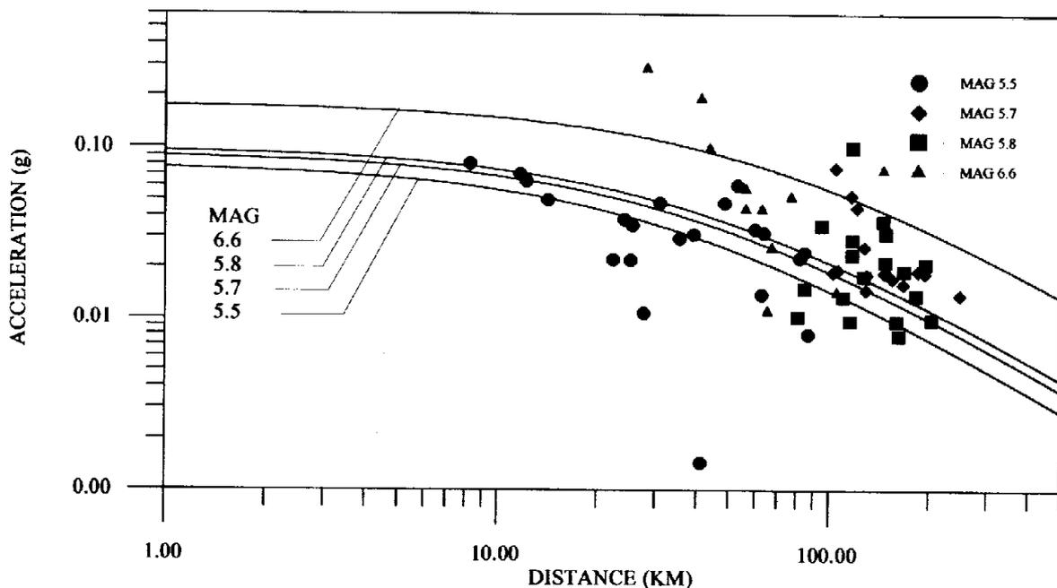
FIG. 3 Proposed new attenuation relationship plotted along with the data set used for the study.
