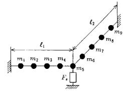
Figure 6: Analytical model of the L-shaped pipe
