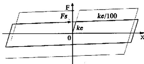
Figure 2: Idealized force-displacement curve of the elastoplastic damper
