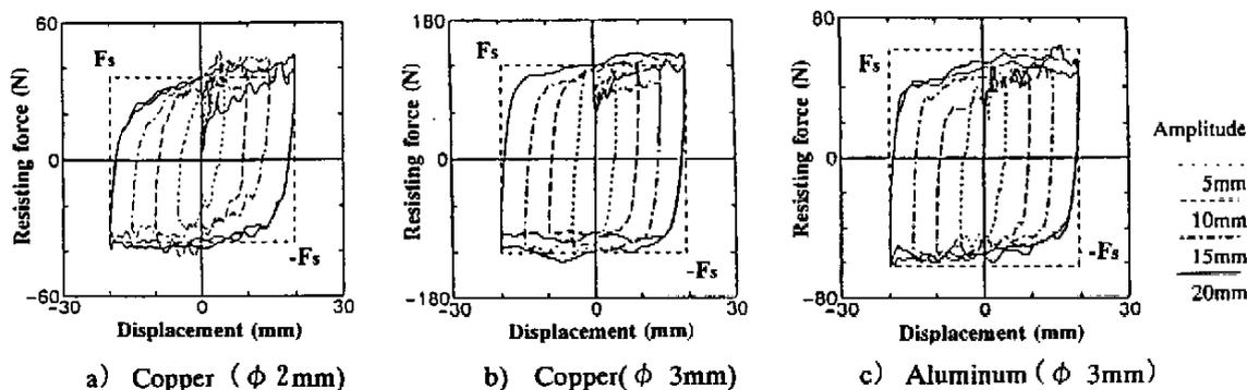
Figure 4: Hysteresis curves of the elastoplastic damper
