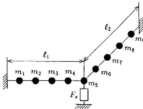
Figure 6: Analytical model of the L-shaped pipe
