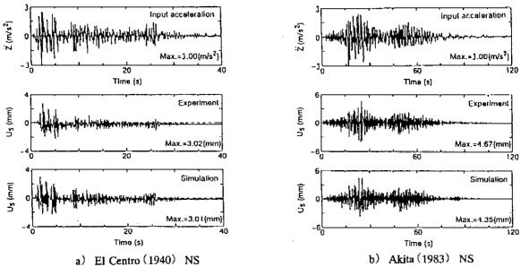
Figure 7: Response deflection waves of the pipe supported by the elastoplastic damper at the corner
