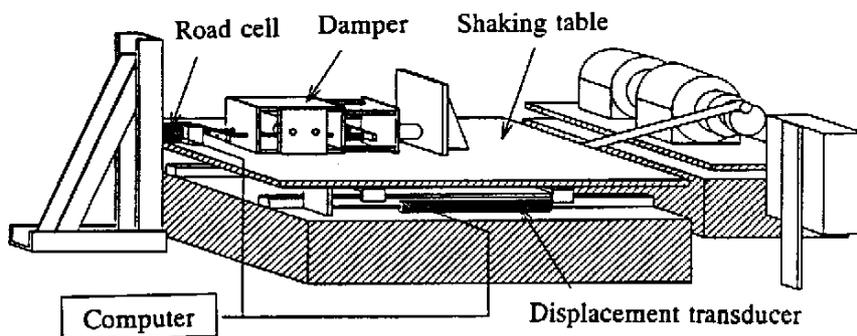
Figure 3: Experimental apparatus
