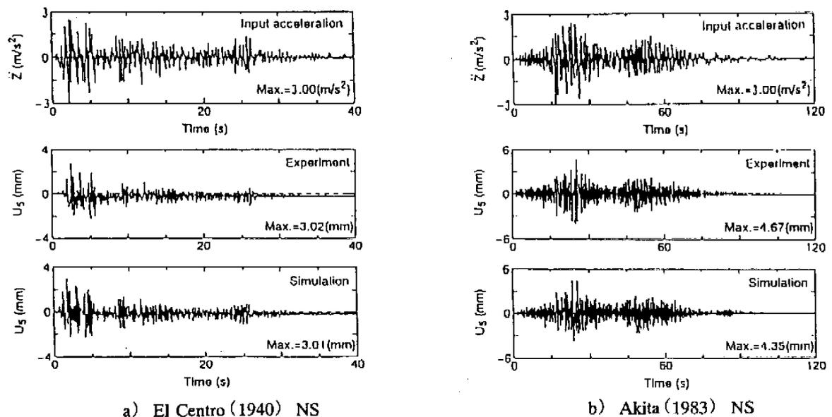
**Figure 7: Response deflection waves of the pipe supported by the elastoplastic damper at the corner**
