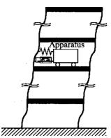
Figure 8: Application of the elastoplastic damper to an apparatus in a building
