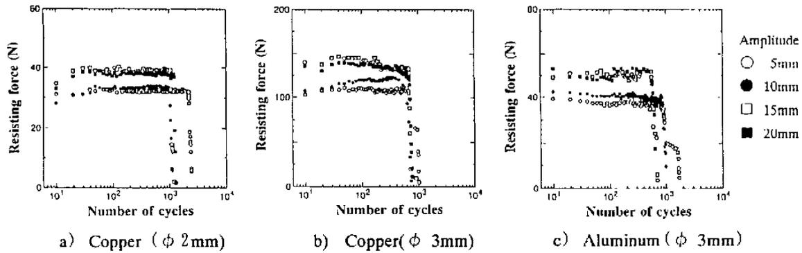
Figure 5: Fatigue life of the rods
