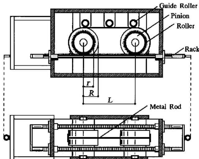
Figure 1: Conceptual sketch of the elastoplastic damper
