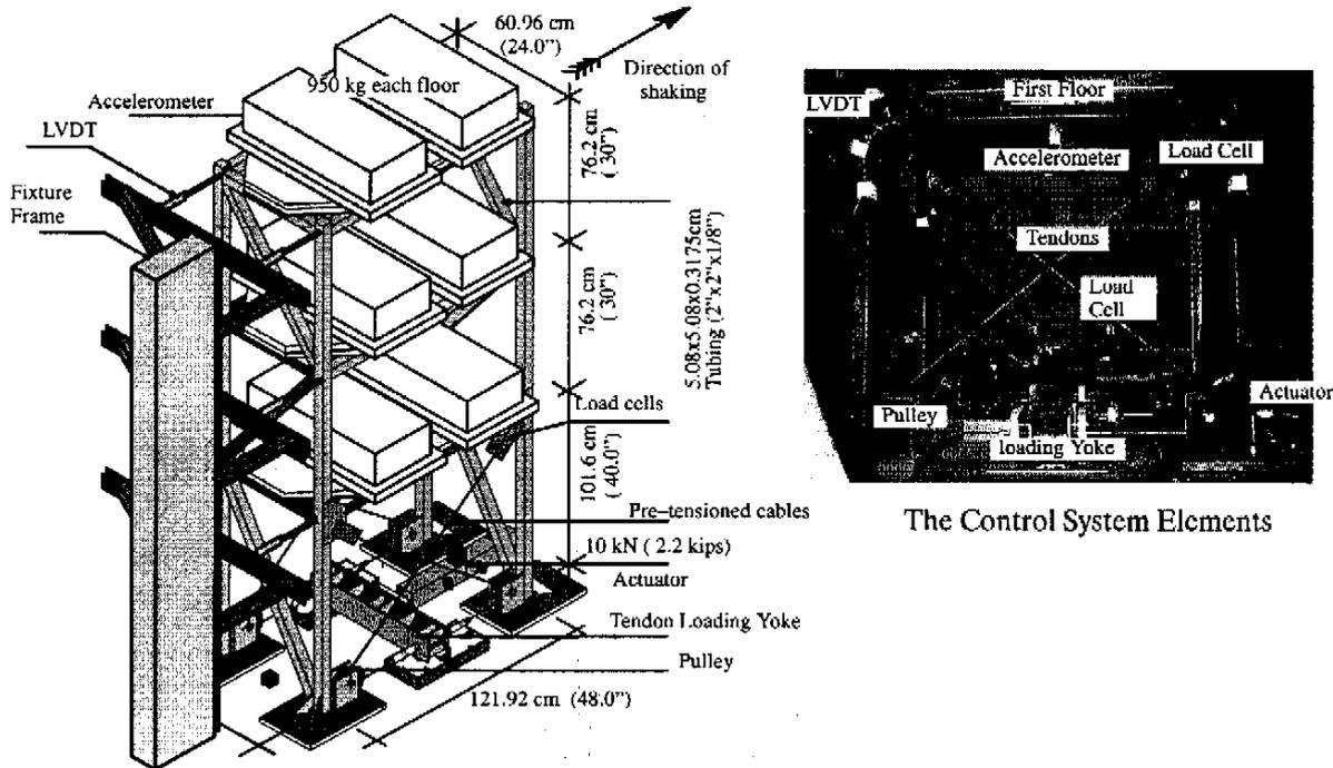
Figure 2. The Test Specimen used in This Study. Three Story Steel Frame with Active Tendons.
