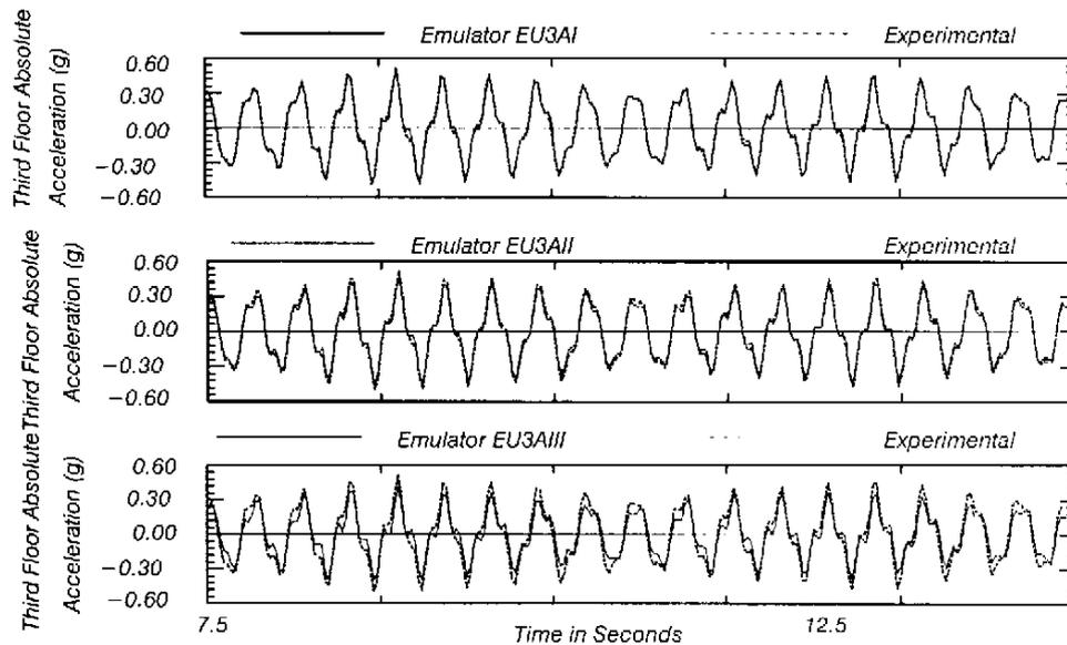
Figure 6. Comparison of the Experimental and Emulators response (using *EU3AI, EU3AII and EU3AIII*). The Structure has been Excited by 50% of Taft Earthquake Record.
