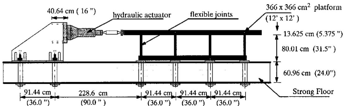
Figure 1. The Earthquake Simulator at the University of Illinois at Urbana–Champaign
