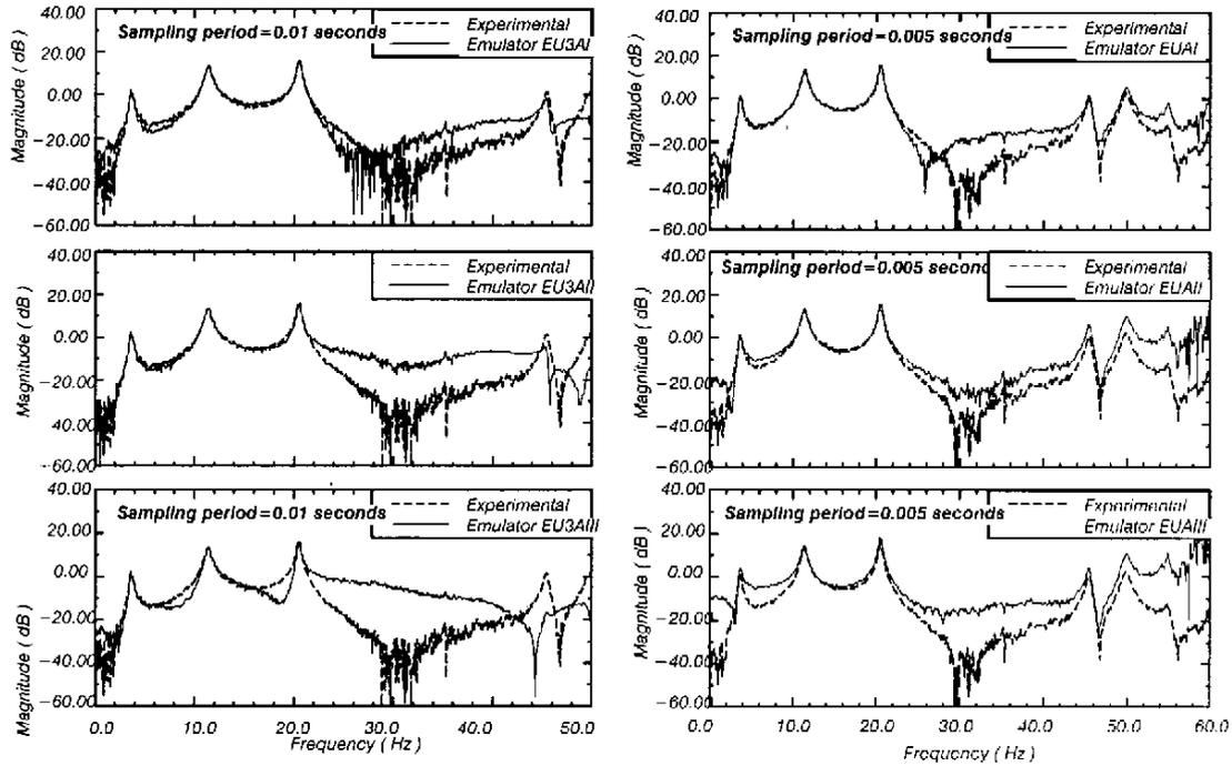
Figure 5. Comparison of the Experimental Transfer Function of the Actuator Command to the *Third Floor Absolute Accelerations* Using both set of the Emulator Neural Networks (*EU3AI, EU3AII, EU3AIII, EUAI, EUAII and EUAIII*).
