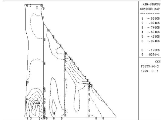
Fig.10:Min.Principle Stress Envelop of Dam
