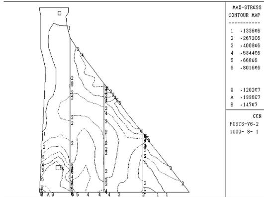
Fig.9:Max.Principle Stress Envelop of Dam
