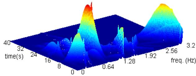
**Fig. 4 Adaptive Spectrogram of Seismic Wave Based on (2)**
