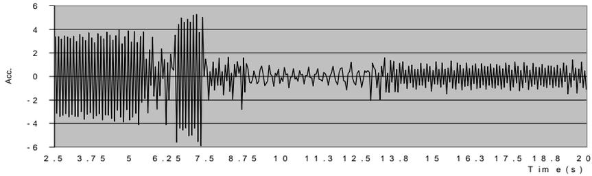
**Fig. 5 Response Acceleration History on Dam Top Based on (1)**
