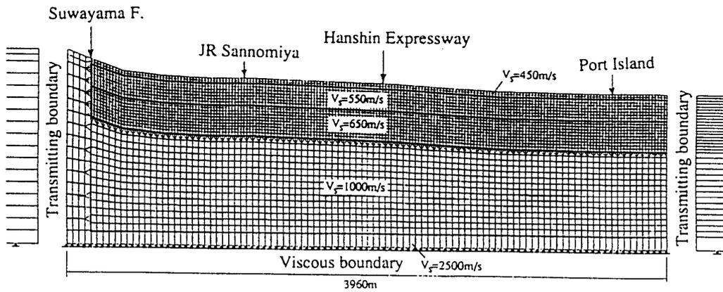
**Figure 3: 2-D FEM soil model (Sannomiya section)**
