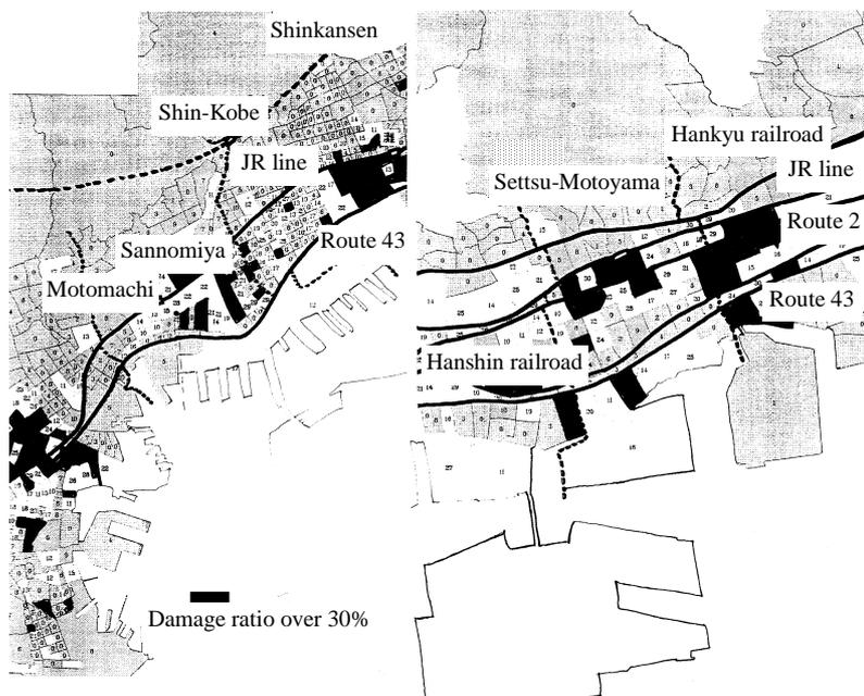
Figure 2: Damage ratio of medium/high rise buildings
