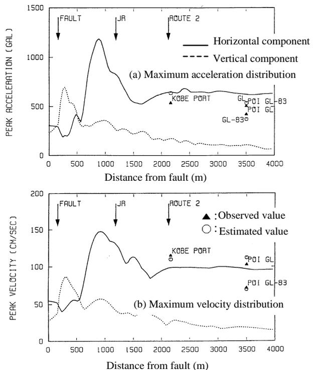
**Figure 4: Maximum acceleration and maximum velocity along Sannomiya section**
