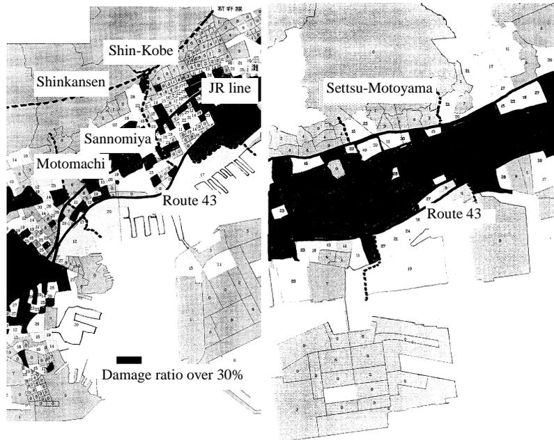
Figure 1: Damage ratio of low-rise buildings
