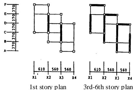
Figure 7: Typical plan of target building
