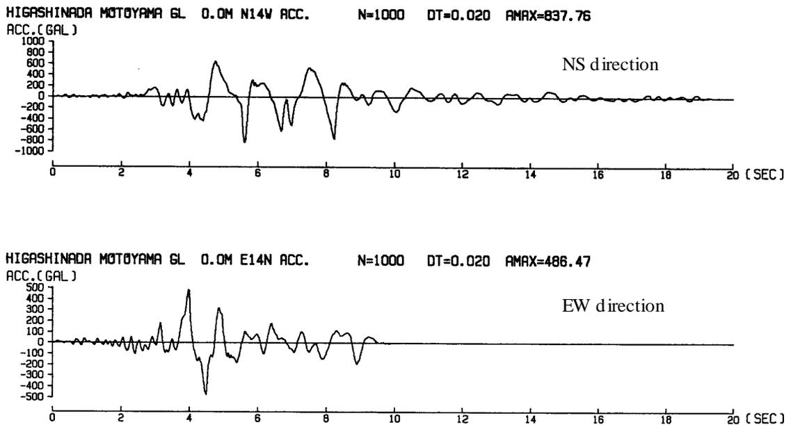
Figure 6: Computed earthquake waves at Motoyama
