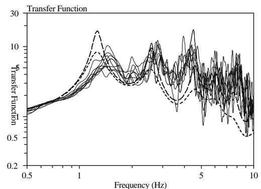
**Figure 7: Fourier spectral ratio at TSUT site**
