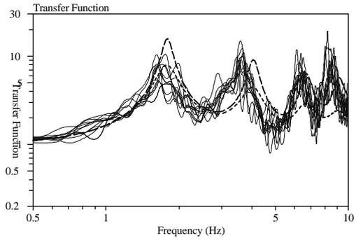
**Figure 9: Fourier spectral ratio at OKIN site**
