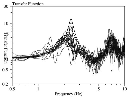
**Figure 3: Fourier spectral ratio at MIYA site**
