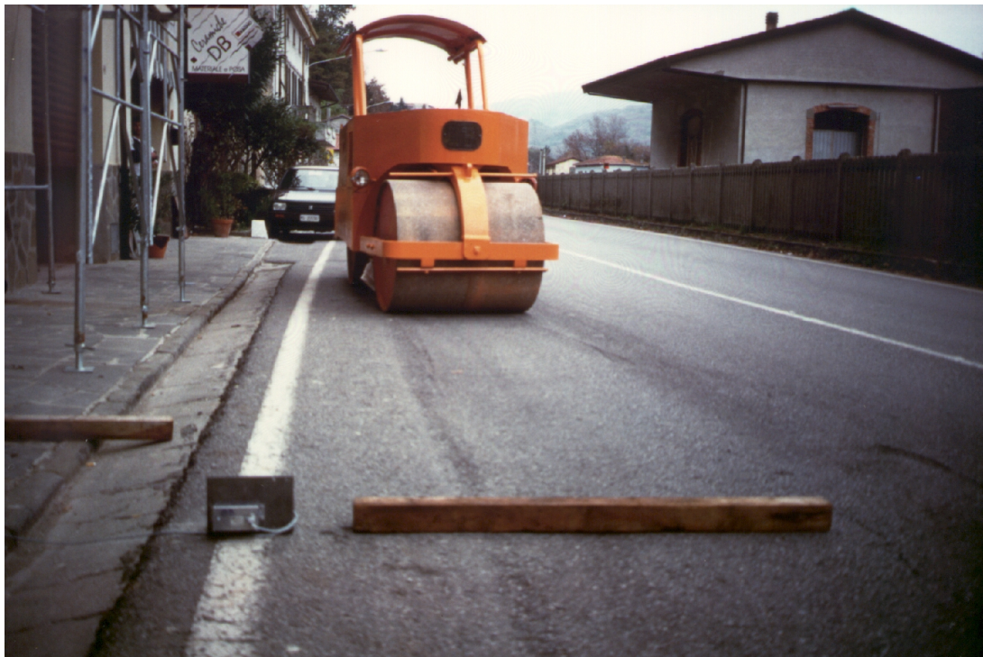
Fig. 1: the road roller in front of the wooden step; on the left of the step an accelerometer can be seen.
