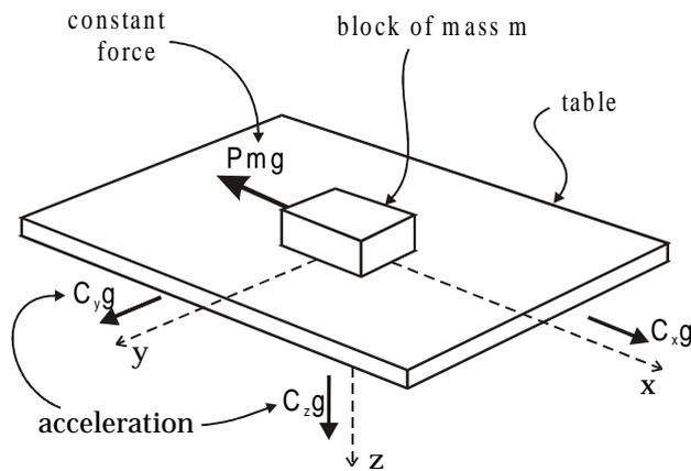
Figure 1 Three-dimensional sliding block model
