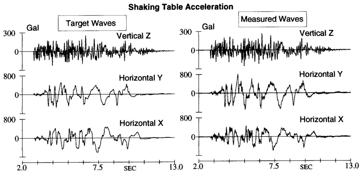
Fig.5 Comparison of acceleration waves at earthquake wave excitation test
