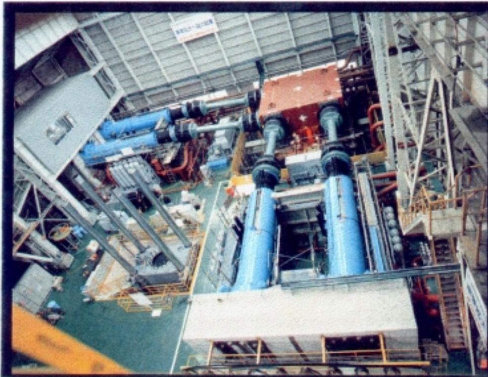
Photo.1 Main part of large actuator test system
