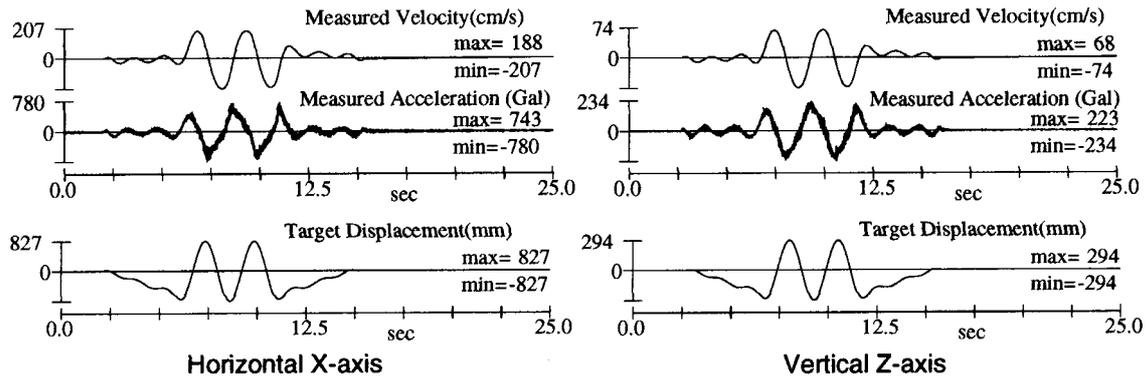
Fig.4 Table response at maximum velocity excitation test
