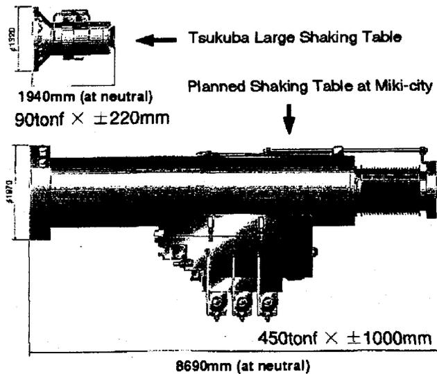
Fig.1 Comparison of horizontal actuator of Tsukuba and the planned new facility
