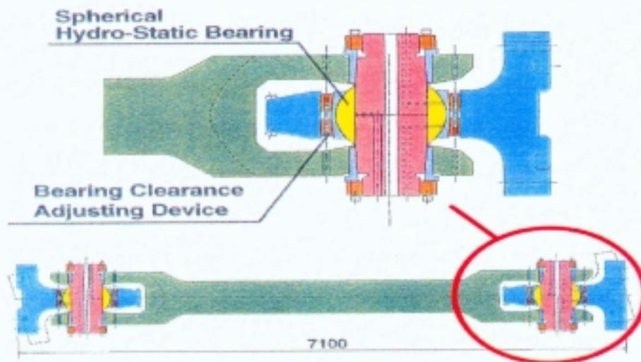
Fig.3 Large 3-D mechanical joint with high pressure spherical bearing
