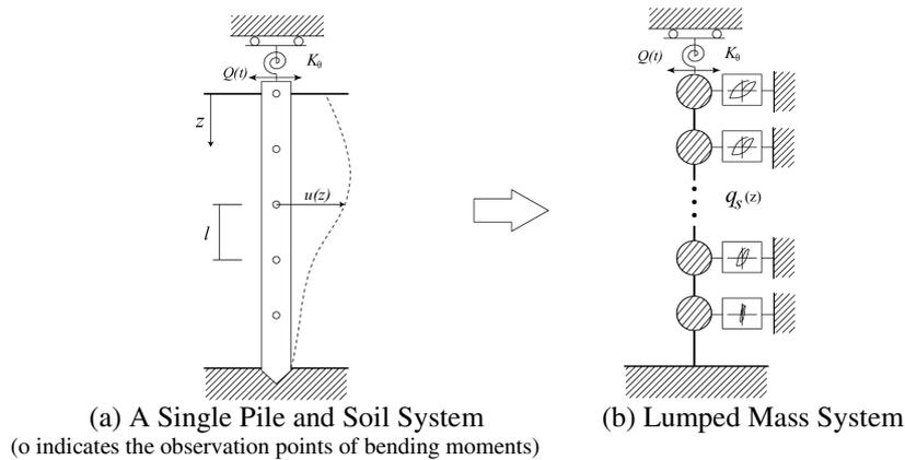
**Fig. 1 Soil-pile system and analysis model**
