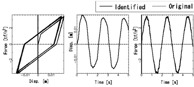
Fig. 2a Estimated results at 2<sup>nd</sup> node without measurement errors (Bi-linear model)
