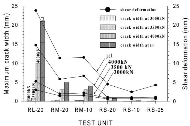
Figure 6 Observed Maximum Shear Crack Width
