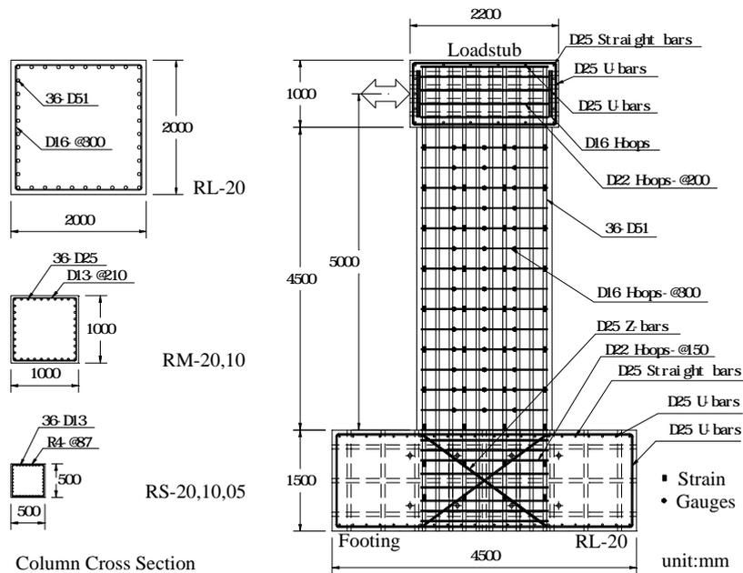
**Figure 1 Reinforcement Details for test columns**
