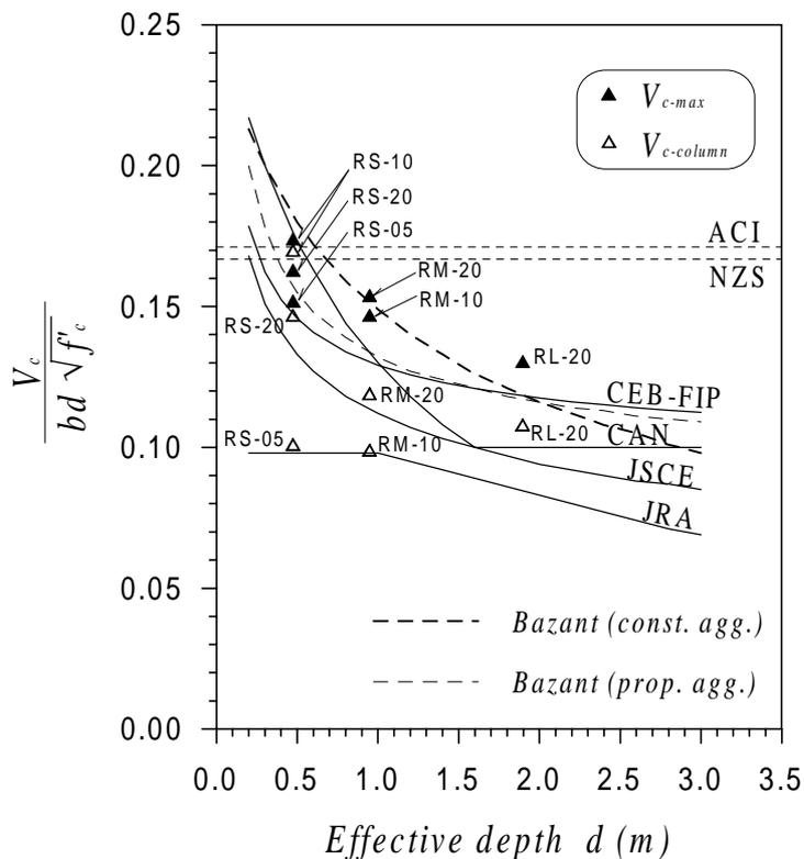
Figure 12 Size Effect on Concrete Shear Component
