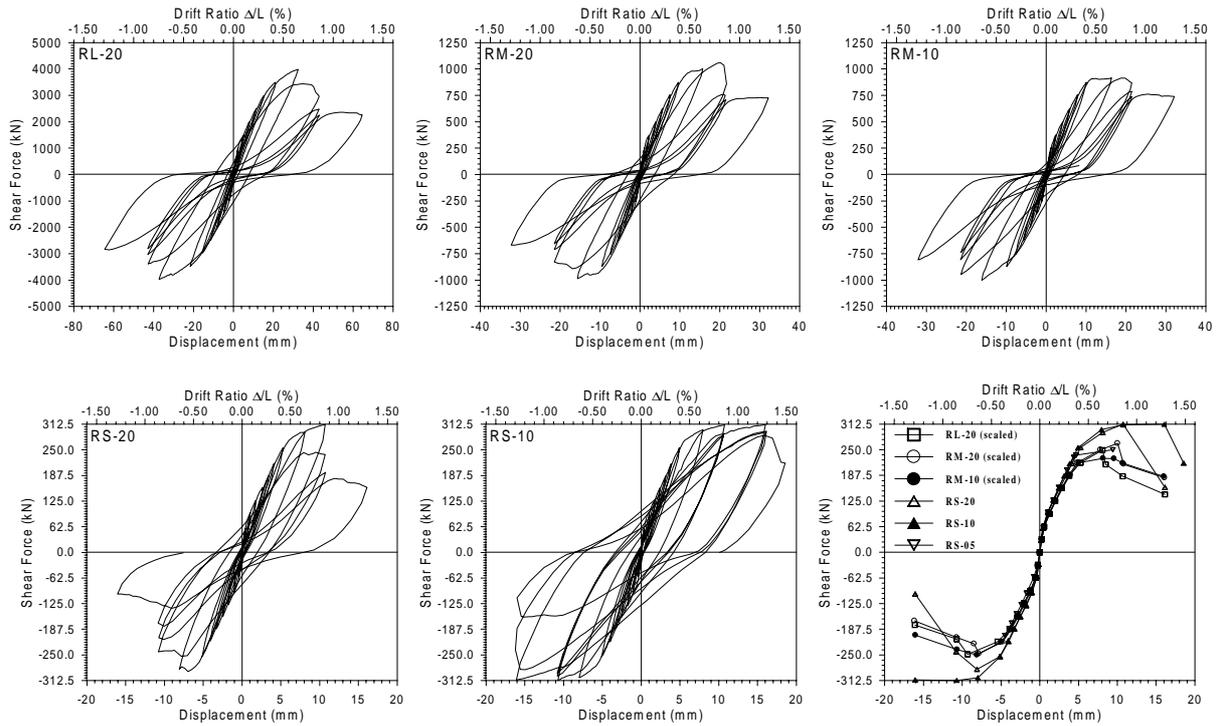
**Figure 7 Hysteretic Response and Comparison of Force Displacement Envelops**
