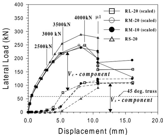
Figure 10 Hoop Shear Component
