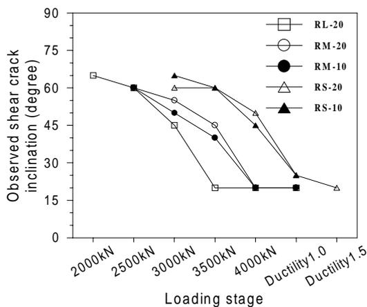
Figure 5 Observed Shear Crack Inclination
