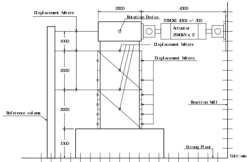
**Figure 2 Column Test Setup for RL-20**
