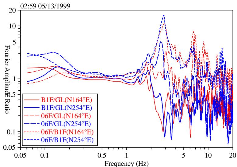
**Figure 6: Fourier Amplitude Ratios B1F/GL, 06F/GL and 06F/B1F at HCH for EQ2**
