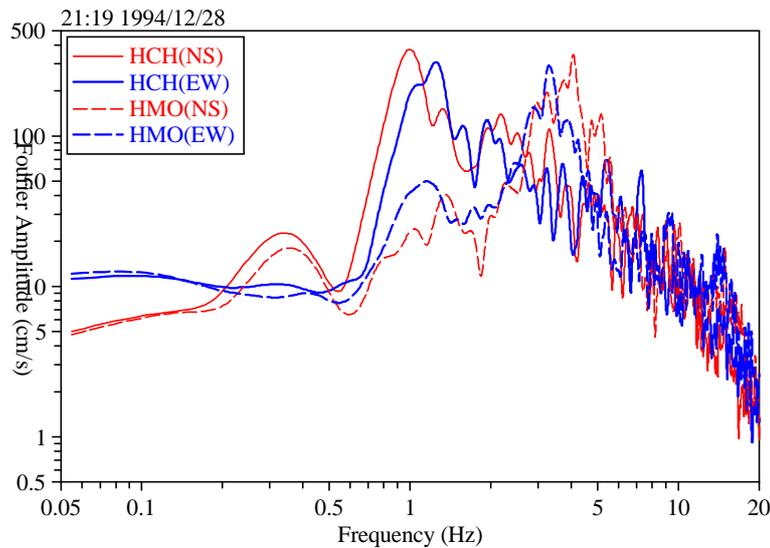
**Figure 2: Fourier Amplitude Spectra of Ground Motions Observed at HCH and HMO for EQ1**
