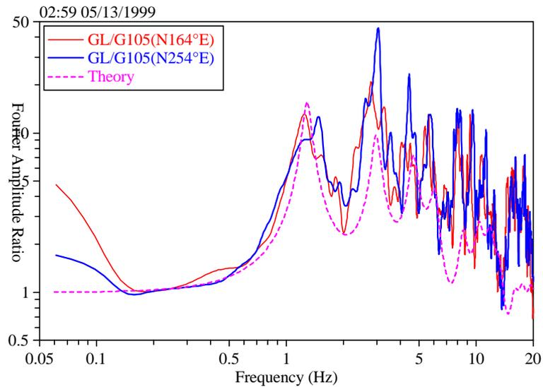
**Figure 4: Fourier Amplitude ratios of Ground Motions at GL to ones at G105 for EQ2**
