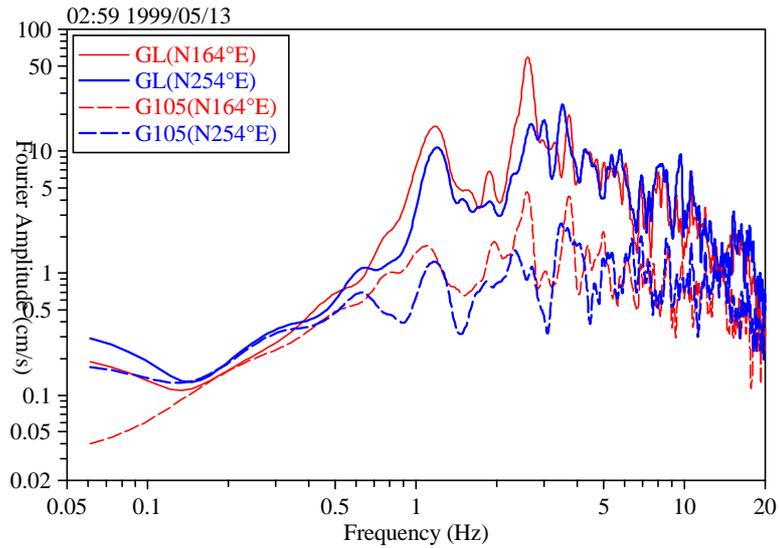
**Figure 3: Fourier Amplitude Spectra of Ground Motions Observed at HCH for EQ2**
