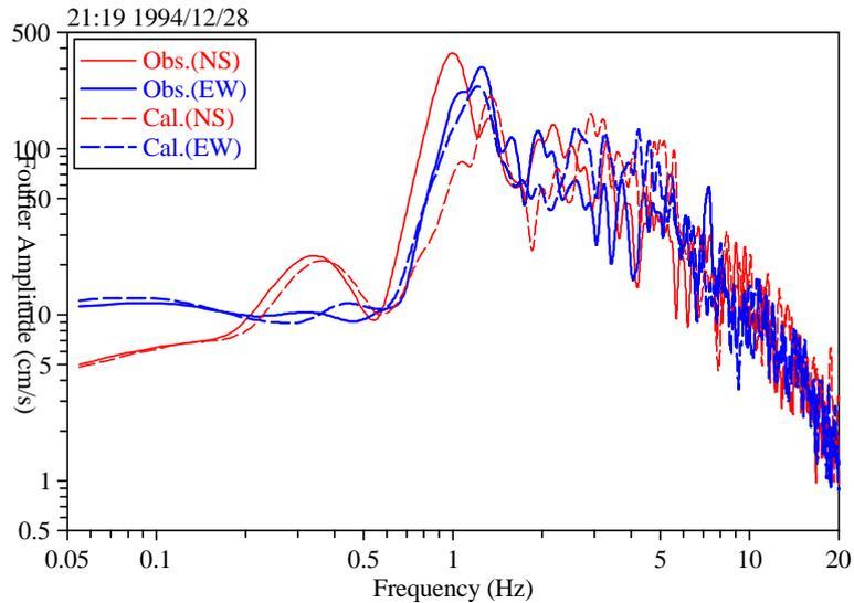
**Figure 5: Fourier Amplitude Spectra of Observed and Calculated Ground Motions at HCH for EQ1**
