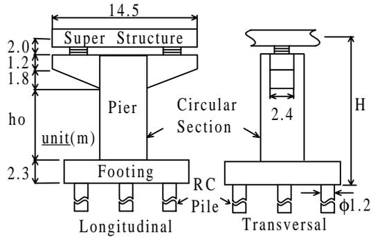
**Fig.1: RC pier with pile foundation**
