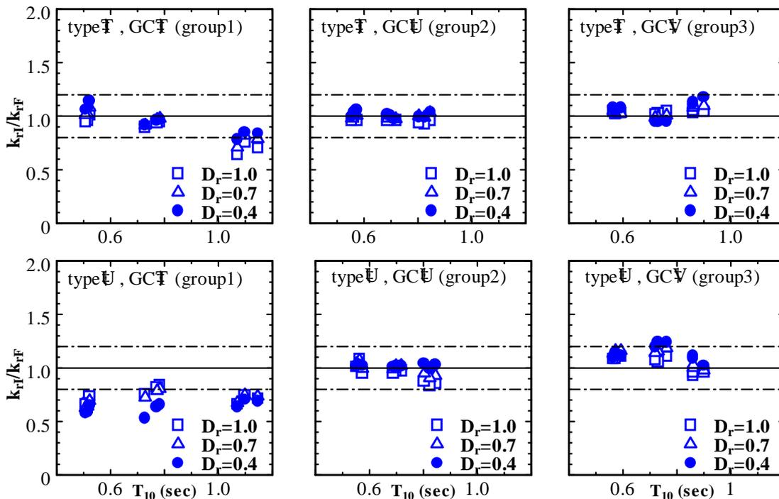
**Fig.7: Ratio of  $k_{rI}/k_{rF}$  of RC piers, comparing the difference in earthquake types (type I, type II) soil conditions (GC= I, II, III) and designated  $D_r$  values ( $D_r=0.4, 0.7, 1.0$ )**
