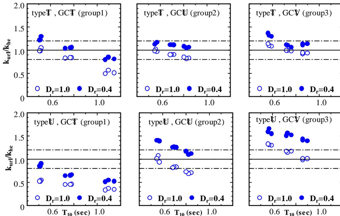
**Fig.8: Ratio of  $k_{ur}/k_{he}$  for pier, comparing the difference in earthquake types, soil conditions and  $D_r$  values**
