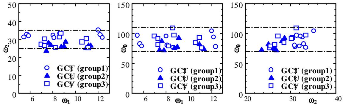
Fig.6: Relationship among natural circular frequencies  $\omega_1$  for pier,  $\omega_2$  and  $\omega_0$  for foundation
