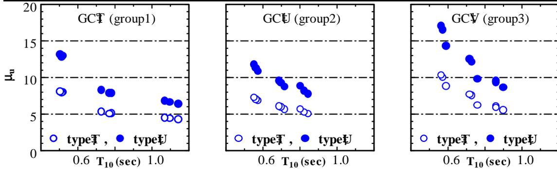
**Fig.4: Relationship between ductility capacity and natural period  $T_{10}$  for RC pier**
