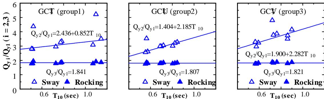
**Fig.5: Ratio of yield strength of  $Q_{y2}$  and  $Q_{y3}(=Q_{y\theta}/H)$  for foundation to  $Q_{y1}$  for pier;  $Q_{y2}/Q_{y1}$  and  $Q_{y3}/Q_{y1}$**
