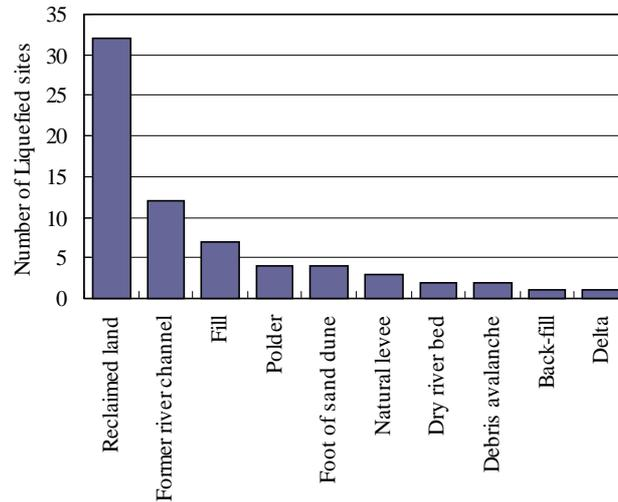
Figure 5: Geomorphological conditions at sites where liquefaction occurred at less than V
