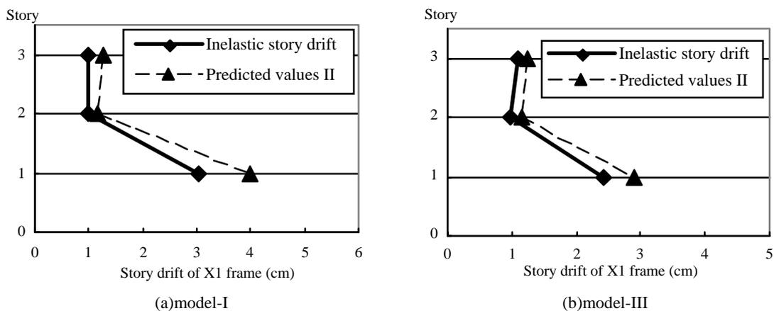
**Figure 12: Prediction of inelastic story drifts at the perimeters in the damage-predicted sides (II)**
