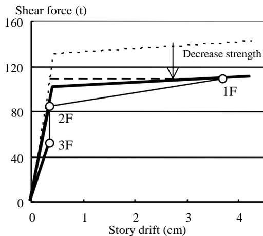
**Figure 8: Modification of the force-deformation relationship for the model-I**
