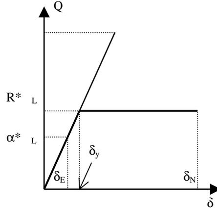
Figure 2: Force-deformation relationship of symmetric system
