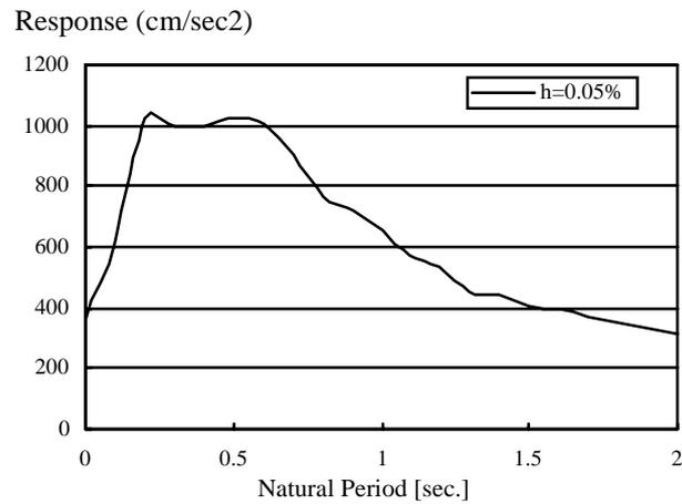
Figure 5: Linear response spectrum
