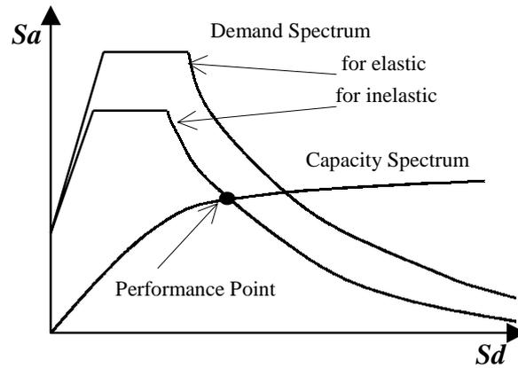
Figure 1 : Capacity Spectrum and demand spectrum
