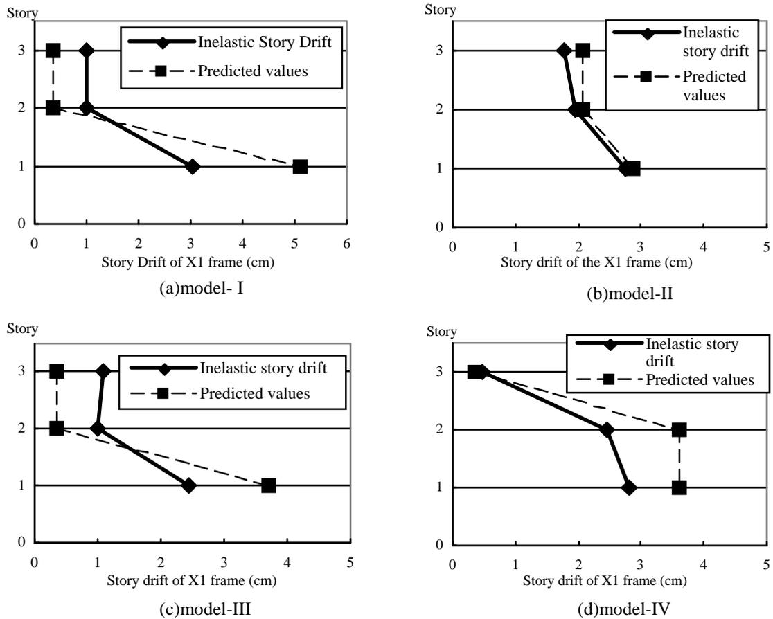
**Figure 10: Prediction of inelastic story drifts at the perimeters in the damage-predicted sides**
