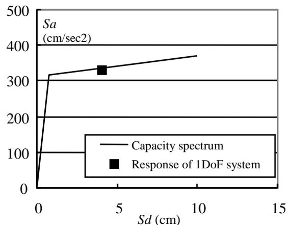
**Figure 9: The capacity spectrum and the inelastic deformation of the equivalent 1-DoF system for the model-I**
