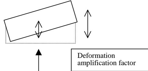
The horizontal seismic design force distribution is supposed to be unchanged still after decreasing the strength capacities. Then story drift distribution can be computed without redoing pushover analysis.
