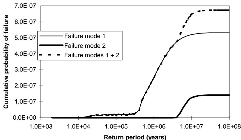
**Figure 4: Cumulative probability function for slender shear wall**
