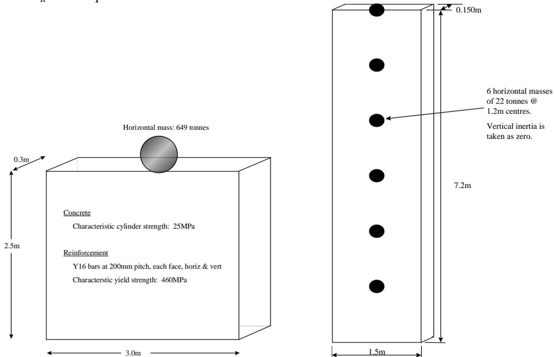
**Figure 2: Geometry of squat and slender shear walls studied**
