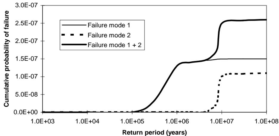
**Figure 5: Cumulative probability function for hypothetical structure**
