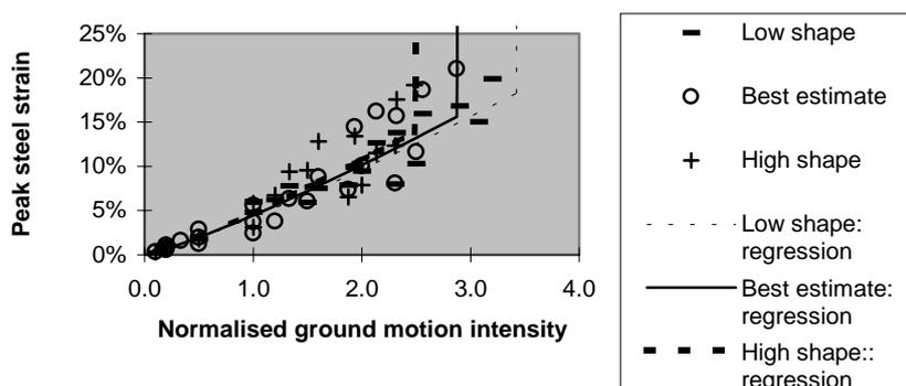
**Figure 3: Regression analysis for slender shear wall**
