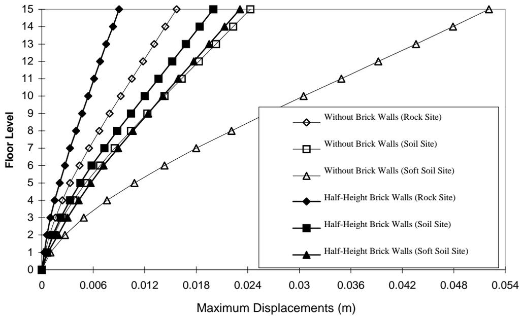
Figure 5: Maximum displacements in the transverse direction of typical building
