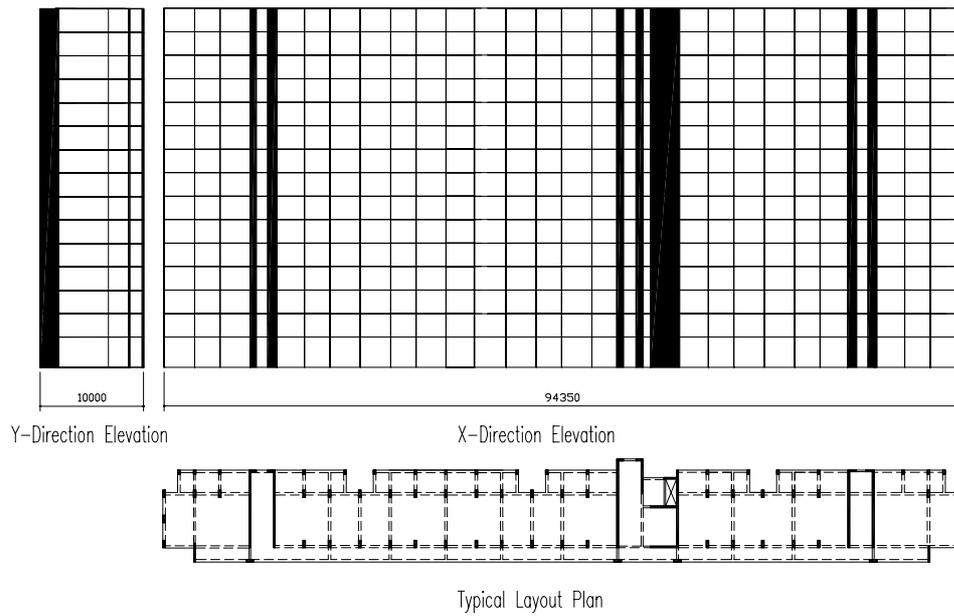
**Figure 3: Elevation views and typical floor plan the typical building**
