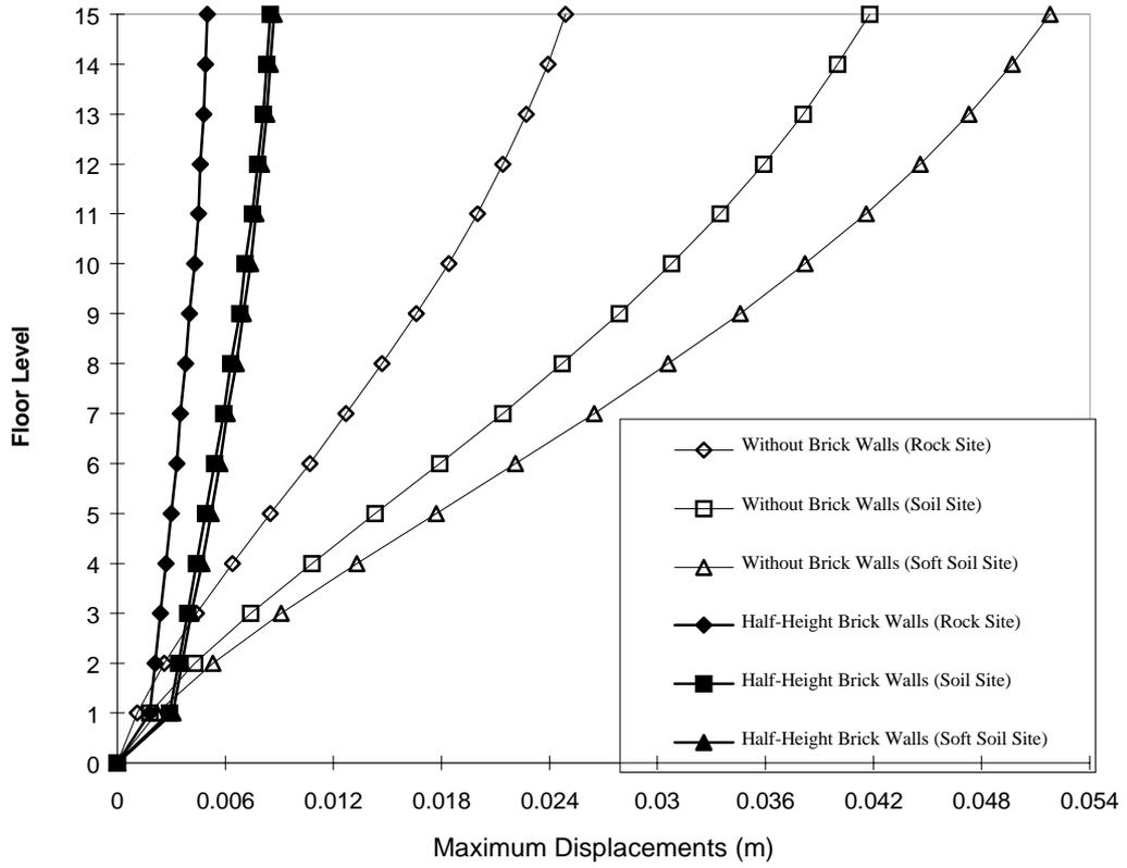
Figure 4: Maximum displacements in the longitudinal direction of typical building
