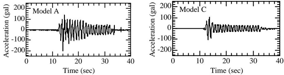
**Figure 9: Acceleration response in the model footing (Models A & C, A6)**
