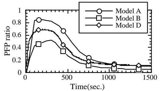
**Figure 12: Pore fluid pressure ratio observed beneath the model footings**
