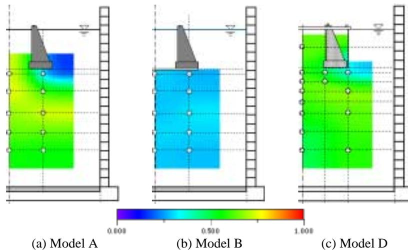
**Figure 15: Contour of pore fluid pressure ratio when the degree of settlement increase dropped** decrease in the rate at which settlement increased. This trend was consistently observed throughout all the tests including the first series in this study.
