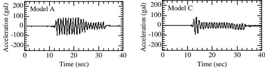
**Figure 8: Acceleration response observed below the center of footing (Models A & C, A9)**
