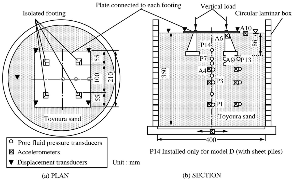
**Figure 3: Schematic figure of centrifuge model**
