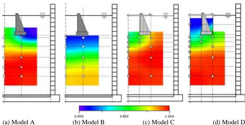
**Figure 14: Contour of pore fluid pressure ratio just after the end of shaking**
