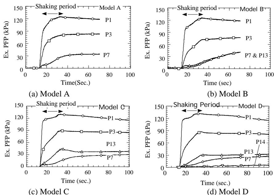
**Figure 11: Pore fluid pressure response observed for Models A - D**
