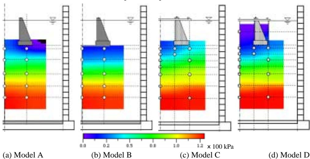
**Figure 13: Contour of pore fluid pressure just after the end of shaking**
