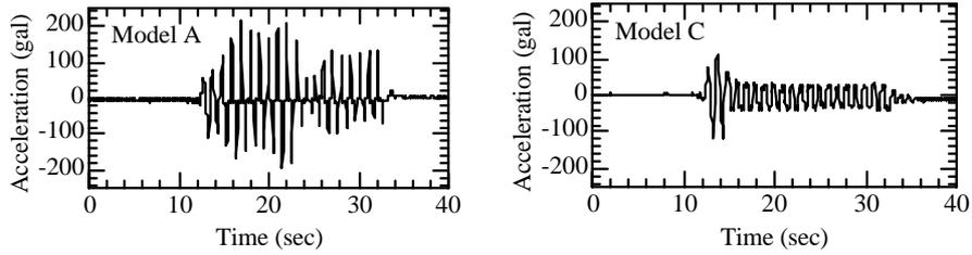
**Figure 7: Acceleration response observed at soil surface (Models A & C, A10)**
