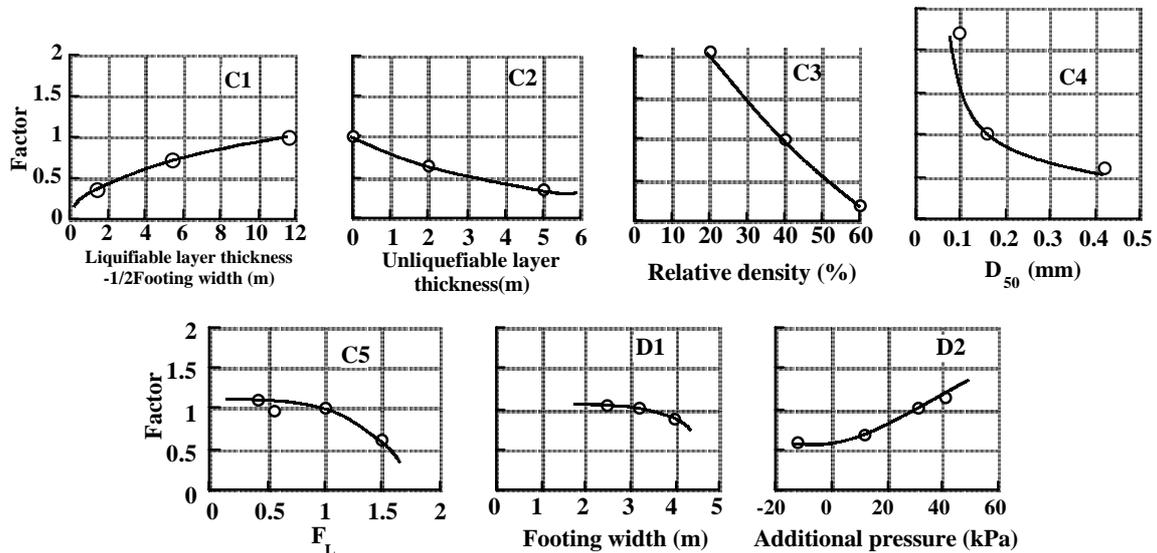
**Figure 2: Deviating factors obtained a series of centrifuge tests**
