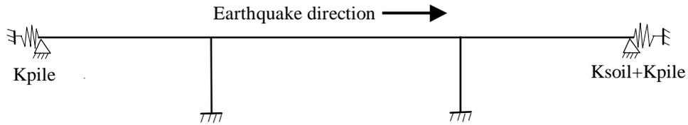
**Figure 3: Abutment stiffness for quasistatic analysis**
