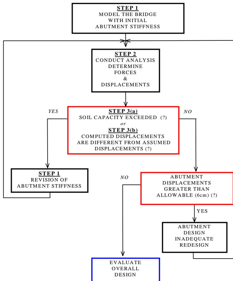
**Figure 4: Schematic presentation of Iterative Analysis Procedure**
