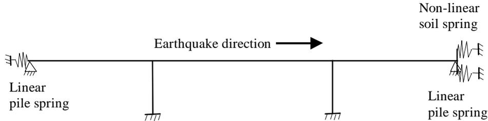
**Figure 7: Abutment stiffness for non-linear static analysis**
