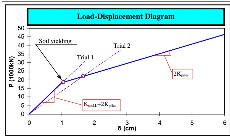
Figure 5: Load-displacement diagram for both abutments in the longitudinal direction
