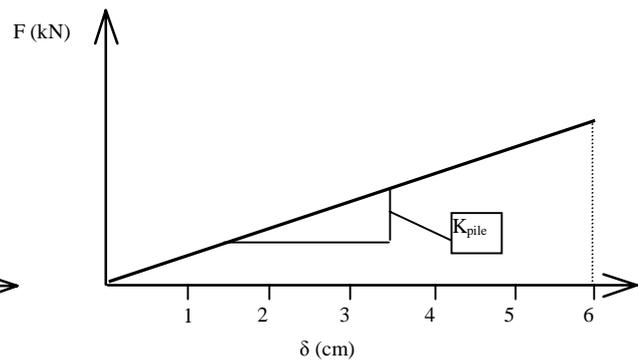
**Figure 9: Linear pile foundation spring**
