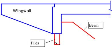
**Figure 1: Monolithic abutment**
