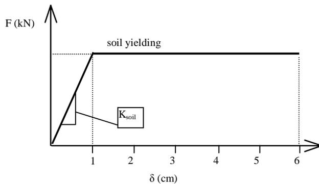
**Figure 8: Non-linear soil spring**
