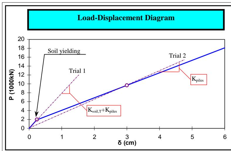
Figure 6: Load-displacement diagram for each abutment in the transverse direction
