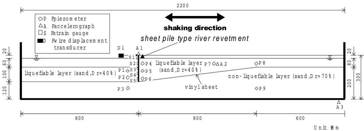
**Fig.2 Soil container and model of the sheet pile type wall**
