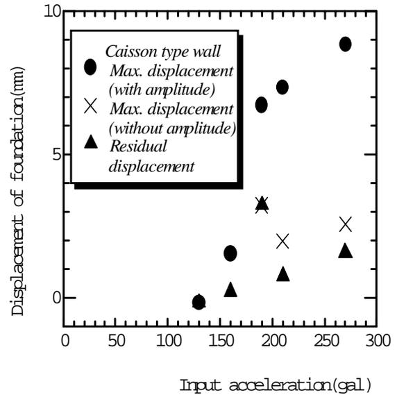
Fig.10 Acceleration vs. displacement of foundation
