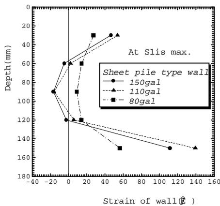
**Fig.14 Distribution of strain of wall**
