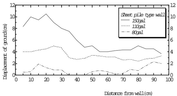
**Fig.15 Distribution of displacement on the ground surface**
