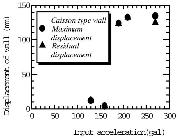
Fig.8 Relationship between displacement of wall and input acceleration
