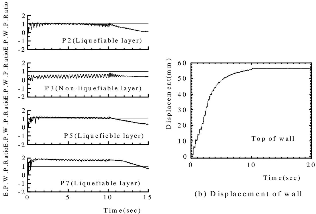
(a) Excess pore pressure ratio
