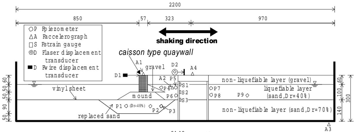
**Fig.1 Soil container and model of the caisson type wall**
