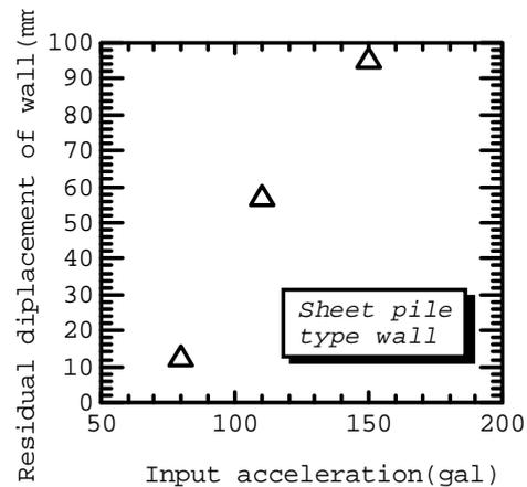
**Fig.13 Relationship between input acceleration and residual displacement of wall**
