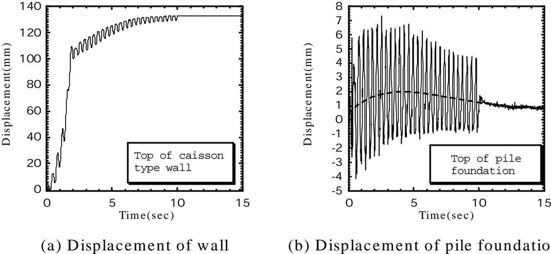
**Fig.3(a),(b) Typical test result for the caisson type wall**
