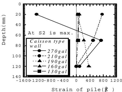
Fig.11 Distribution of strain of pile in depth
