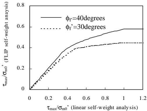
**Figure 3: Shear stress ratio resulting from self-weight analysis by FLIP versus shear stress ratio resulting from linear self-weight analysis**
