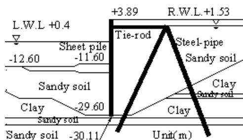
Figure 1: Cross sectional view of quay wall A of Osaka port
