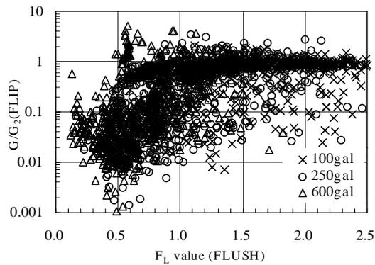
**Figure 4: Quay wall A at Osaka Port:  $G/G_2$  versus  $F_L$**
