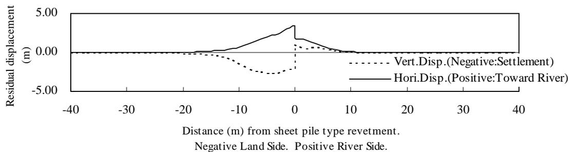
**Figure 13: Distribution of horizontal and vertical residual displacements on soil surface and riverbed**
