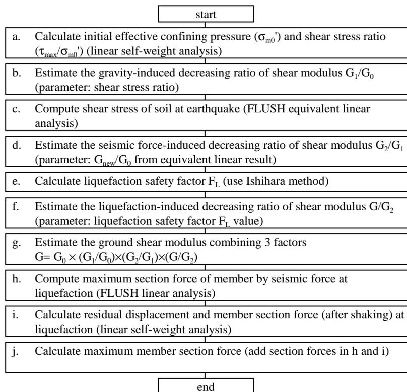
Figure 7: Calculating procedure for FLUSH-L method
