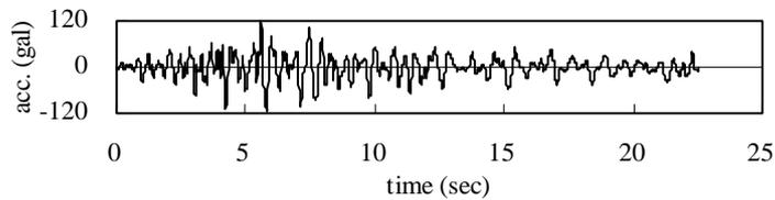
**Figure 10: Seismic wave for input (modified wave from one observed by Akita Prefectural Government at 1964 Niigata earthquake)**
