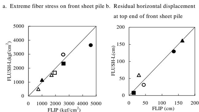
Figure 2: Comparison of results by FLUSH-L method and FLIP for quay wall A (■□), coastal levee B (●○) and revetment C (▲△) at Osaka Port ■●▲: Current cross section. □○△: Improved cross section. Seismic wave for input: Hachinohe wave (max. acceleration 250 gal).
