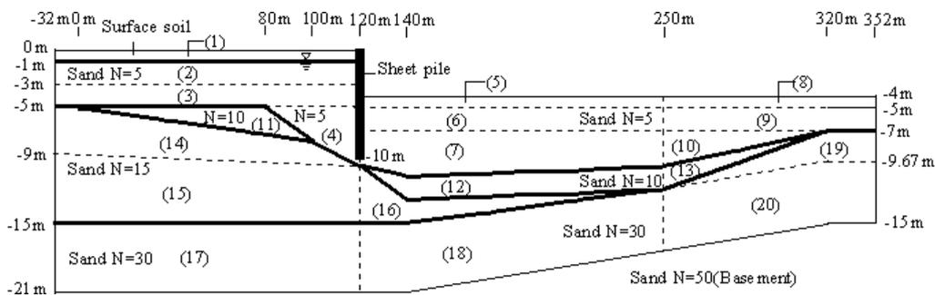
**Figure 8: Soil Layer divisions (ordinate is magnified 10-fold with respect to abscissa). (1) to (20) are material numbers.**
