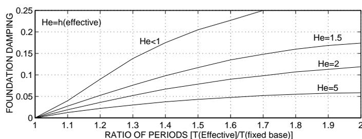
**Figure 7. Foundation damping [adopted from ATC3-06 , 1978 and Veletsos , 1977].**
