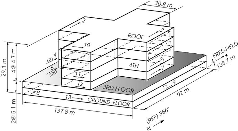
**Figure 1. Three dimensional schematic of OVH building and seismic sensor locations**
