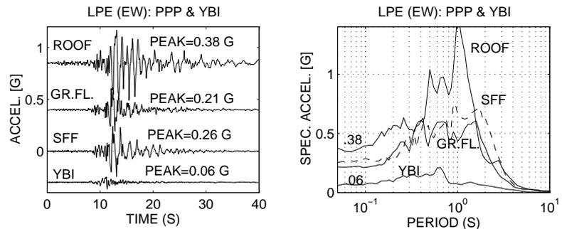
**Figure 5. Recorded (EW) accelerations and corresponding response spectra at the free-field, ground floor and roof of Pacific Park Plaza (PPP), and at Yerba Buena Island (YBI) [at approximately the same distance as PPP] depict the level of amplification at PPP site.**
