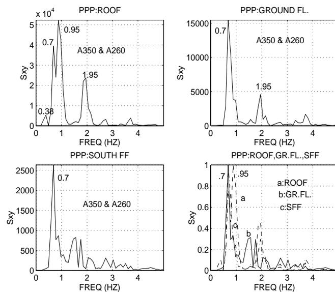
**Figure 6. Cross-spectra of orthogonal accelerations (A350 & A260) at the roof, ground floor, free-field of PPP. Also shown (bottom right) is the normalized cross-spectrum depicting structural and site frequency peaks. (350 & 260 depict degrees clockwise from true north).**
