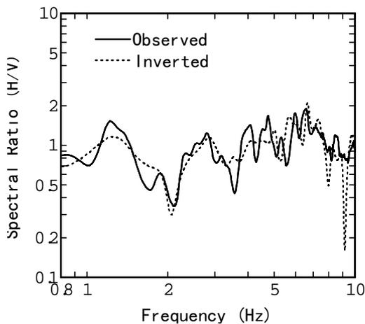
Figure 9: Comparison of spectral ratios in the inversion at Tomioka site
