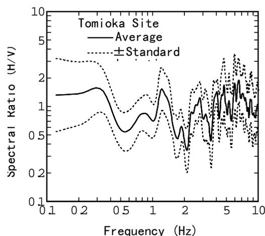
**Figure 7: Observed spectral ratio at Tomioka site**
