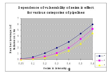
Figure 3: Dependence of vulnerability of seismic effect for various categories of pipelines
