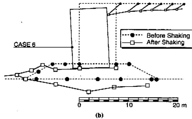
Figure 5 Residual displacement of model quay walls (scaled in terms of prototype)
