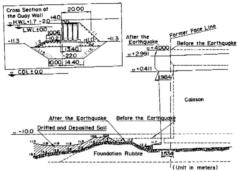
Figure 6 Deformation of rubble mound beneath the caisson (measured by diving)
