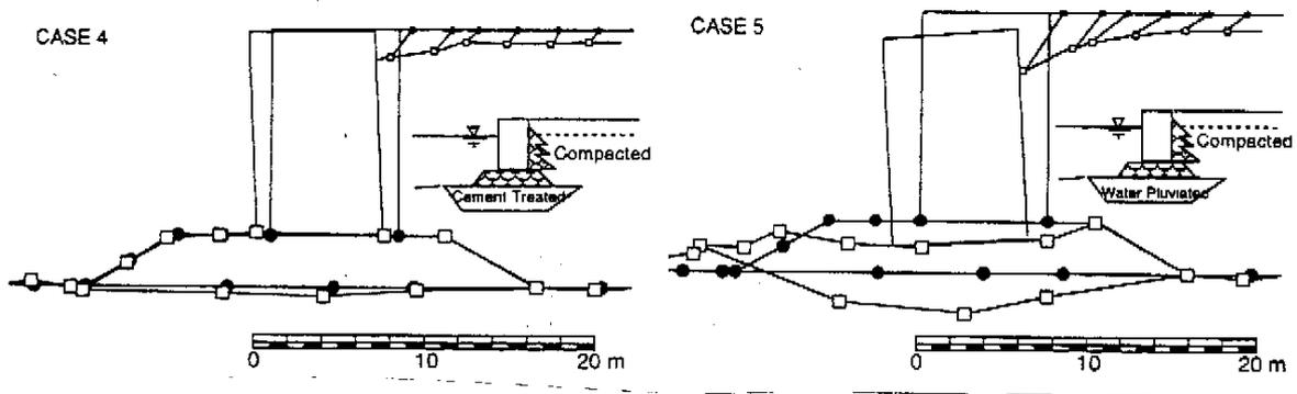
(a) Deformation of foundation rubble and ground surface (Cases-4 & 5)
