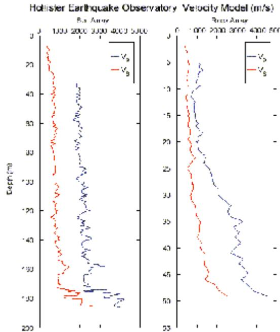
**Figure 7. Measured velocity profiles from the HEO main soil station and remote rock station.**
