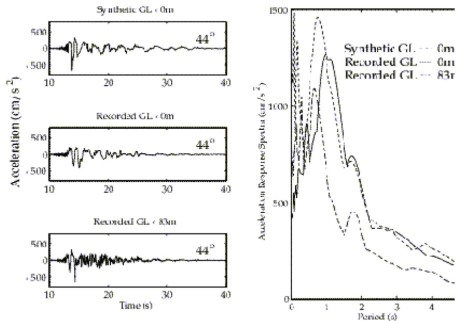
**Figure 9. Ground motion prediction at PI. The Hyogo-ken Nambu (Kobe) earthquake surface soil ground motion (44° component) is modeled using the observed GL-83 as the input motion. Comparison of the time history (left) and 5% damped response spectra (right) is shown.**
