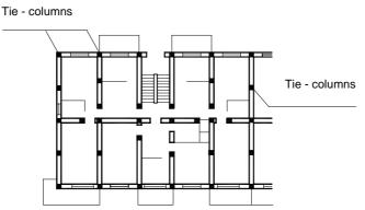
Figure 6 : Layout of tie-columns on the ground floor
