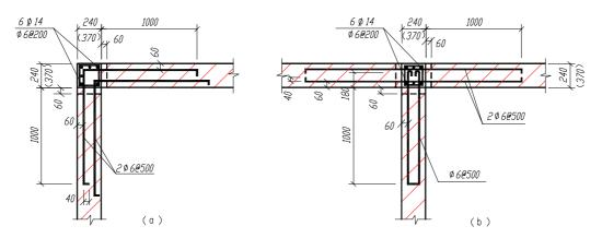
Figure 7 : Construction details of terminal tie-columns
