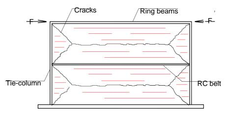
Figure 2 : Cracks on the wall panel strengthened with RC belt
