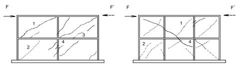
Figure 3 Cracks on the wall panel with 3 RC Tie Columns.
