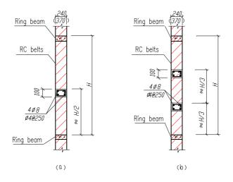
**Figure 10 : Joints of the reinforced concrete ring beams**
