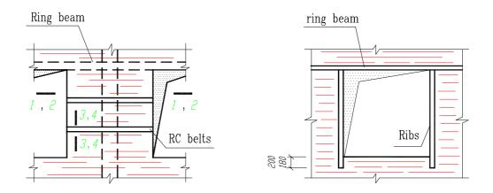
Figure 11 : RC belts on walls Between windows Figure 12 : RC edge ribs of walls between windows
