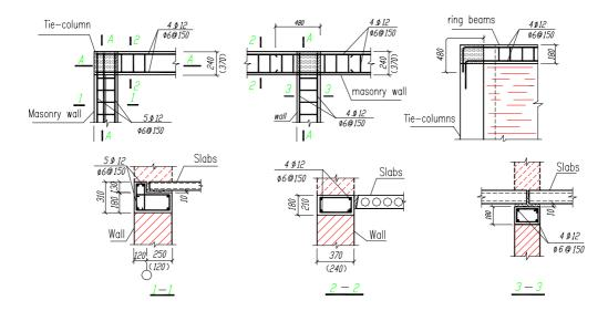
Figure 9 : Joints of the reinforced concrete ring beams
