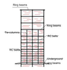
Figure 5 : Vertical cross section of 8-storied confined masonry building
