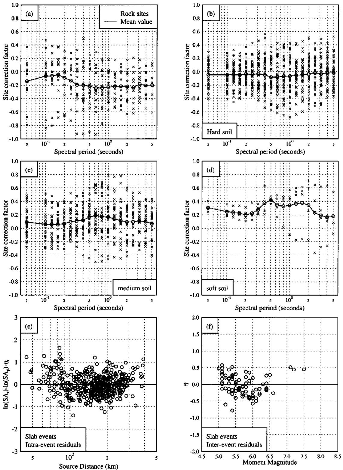
Figure 3 Variation of site correction factors and their mean values with periods and residual distributions, (a) rock sites; (b) hard soil sites; (c) medium soil sites; (d) soft soil sites; (e) intra-event residuals; and (f) inter-event residuals. Parameters for PGA are plotted at 0.05s for plotting convenience.
