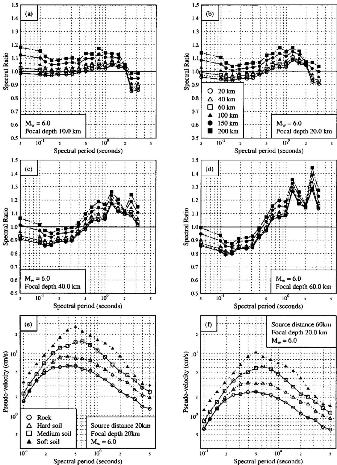
Figure 4 Spectral ratio between the model for the western part of Japan and that for all Japan and the pseudo-velocity spectra predicted by the model for all Japan for  $M_w = 6$  (a) 10km depth; (b) 20km depth; (c) 40km depth; (d) 60km depth; (e) 20km source distance; and (f) 60km source distance. Parameters for PGA are plotted at 0.05s for plotting convenience.
