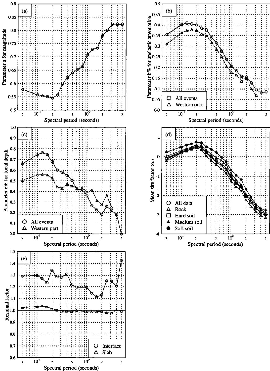
Figure 2 Model parameter variation with periods for all events, and the western part of Japan and residual factors, (a) parameter a for magnitude; (b) parameter b for anelastic attenuation term; (c) depth term; (d) mean site factors; and (e) residual factors for interface and slab events. Parameters for PGA are plotted at 0.05s for plotting convenience
