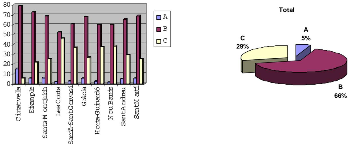
**Figure 5. Vulnerability classes of the buildings for the 10 districts of Barcelona and for the complete city. (See explanations in the text).**
