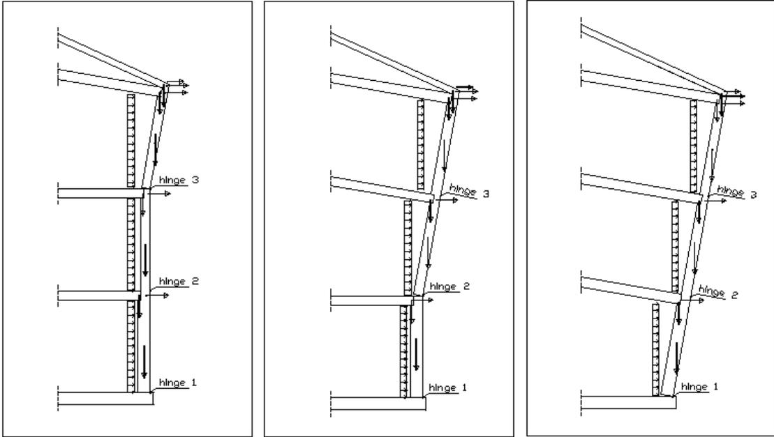
**Figure 1: Selection of the possible overturning configurations**
