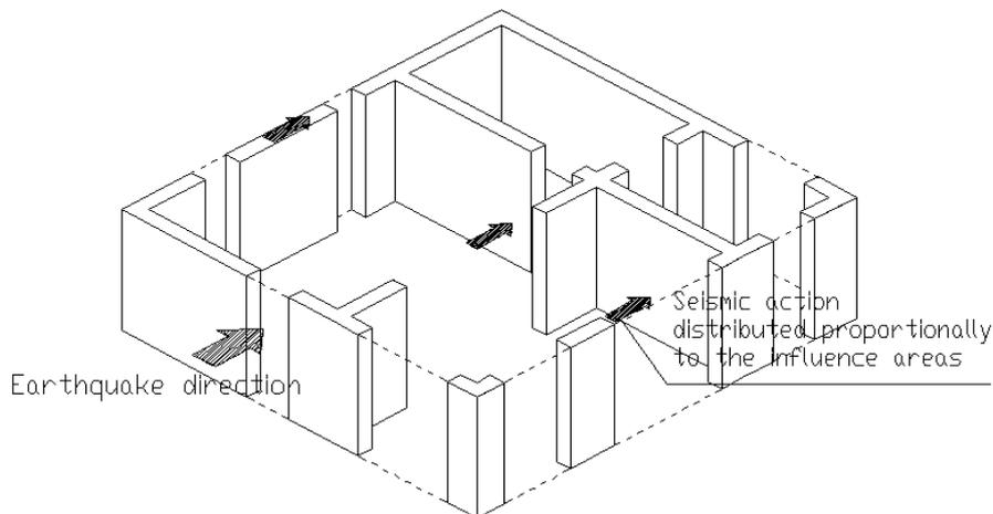
**Figure 5: Distribution of the seismic forces with the deformable floors option**
