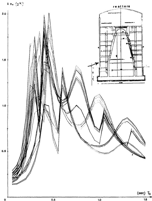
Fig. 2: Example of floor response spectra at a point of a reactor building. Two different soil conditions two different damping distributions, and 9 different models for the structure are considered. Ground acceleration .2 g.
