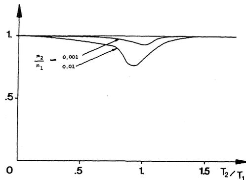
Fig. 4 Reduction for  $A = \frac{\ddot{S}_2}{\ddot{S}_1}$  due to feedback from  $m_2$  to  $m_1$ .
