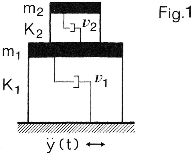
The elementary model obtained by applying modal analysis independently to the building and to equipment.
