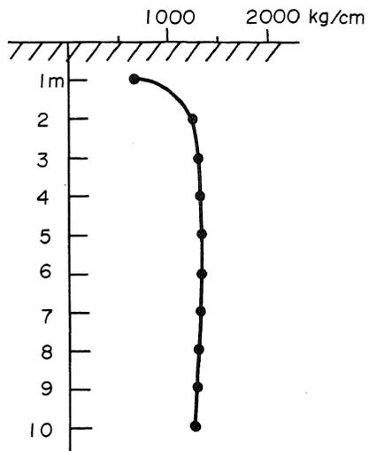
Fig. 14 Dynamic Spring Constants of the Ground
