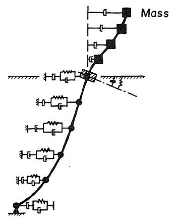
Fig. 6 Lumped Mass System for a Pile Foundation
