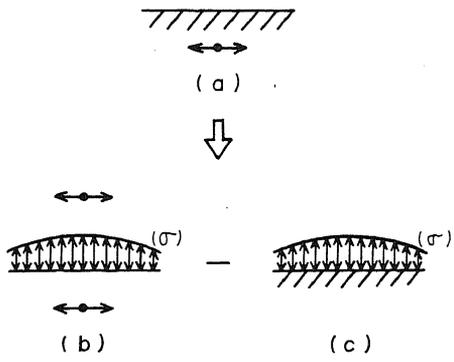
Fig. 7 Two Stages for Obtaining Solution of One Point Excitation in Elastic Half Space
