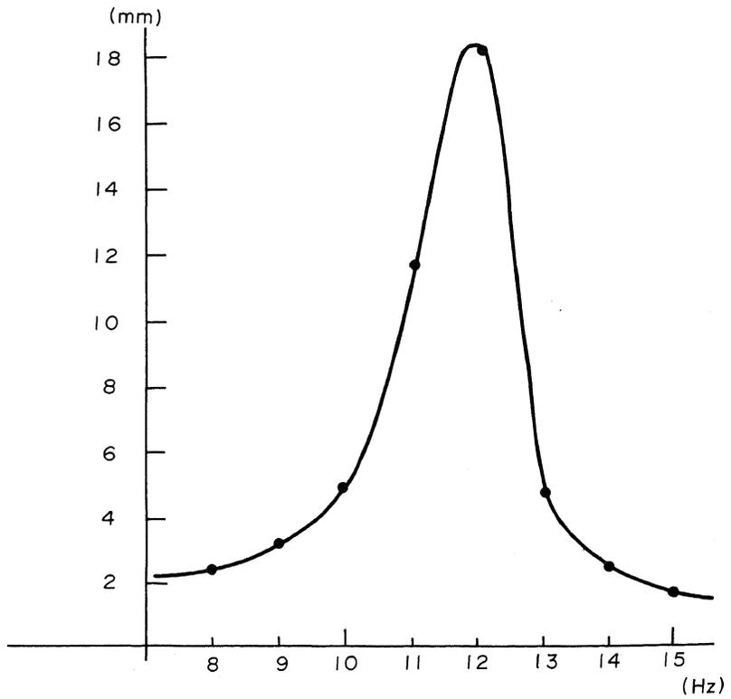
Fig. 16 Computed Resonance Curve of a Pile Foundation
