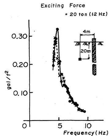
Fig. 4 Resonance Curve of Pile Foundation of Field Tests
