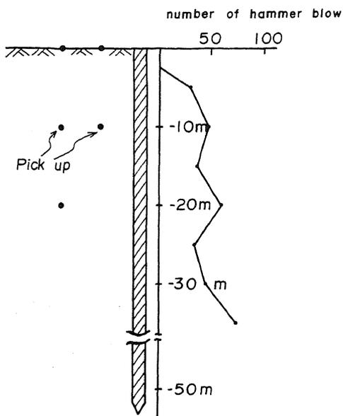
Fig. 1 Soil Condition of Pile Foundation
