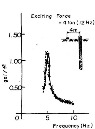
Fig. 2 Resonance Curve of Pile Foundation at Field Tests
