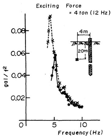
Fig. 3 Resonance Curve of Pile Foundation at Field Tests
