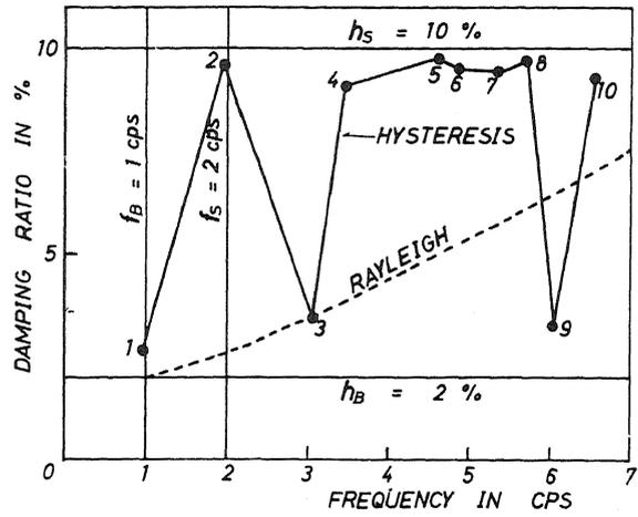
Fig.2 Relationship between frequency and damping ratio
