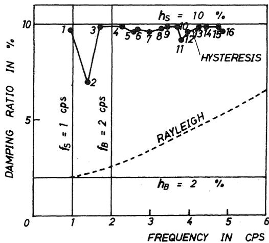
Fig.5 Relationship between frequency and damping ratio
