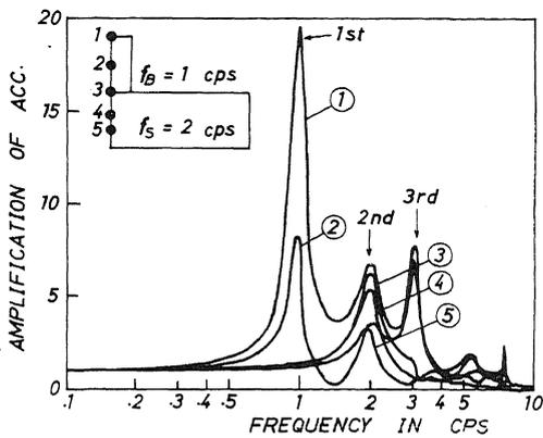
Fig.3 Magnification factor of acceleration
