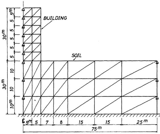
Fig.1 Finite element idealization
