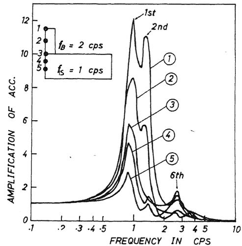
Fig.6 Magnification factor of acceleration
