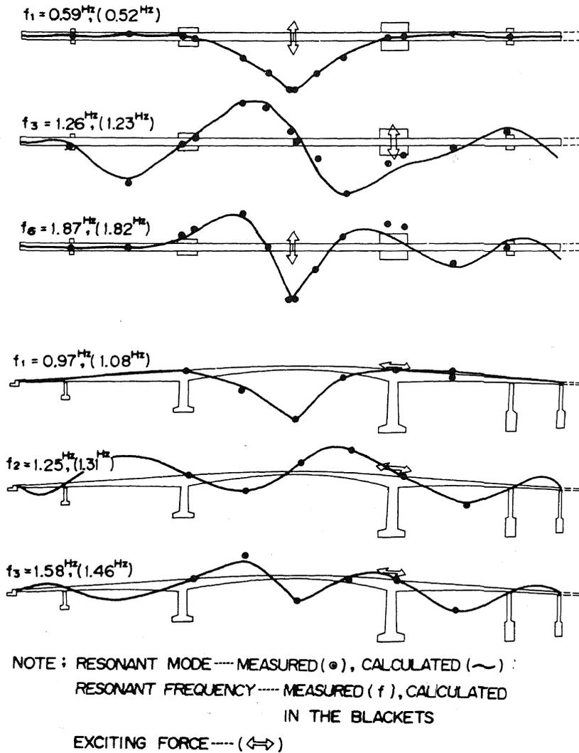
Figure-3 Examples of Resonant Mode and Frequency
