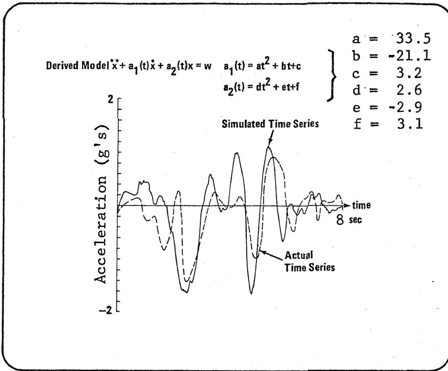
Fig. I El Centro South Earthquake - Comparison of Simulated and Actual Record
