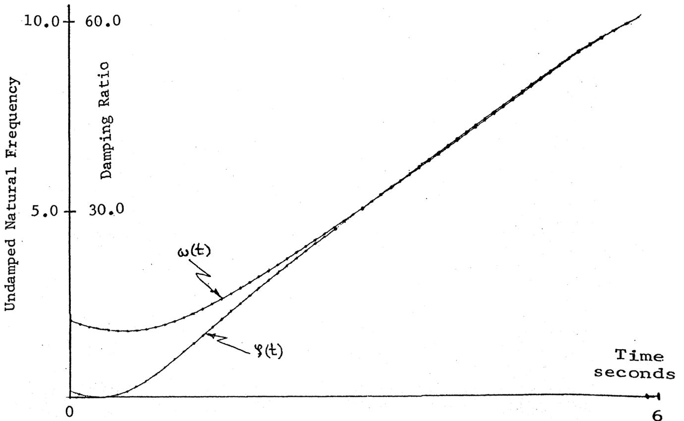
Fig. II Undamped Natural Frequency ( $\omega$ ) and Damping Ratio ( $\zeta$ ) vs. Time
