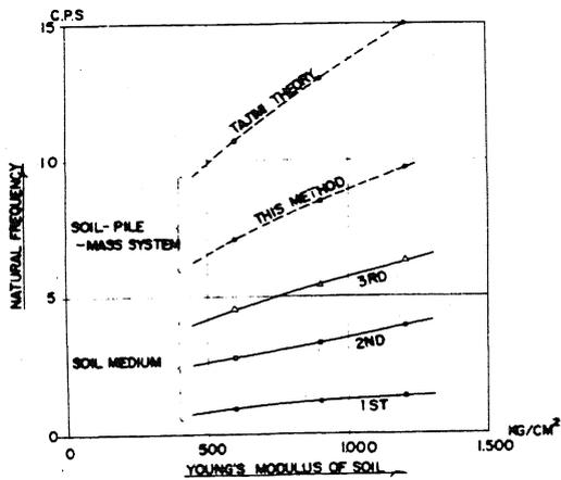
Fig. 3 Comparison between Tajimi's theory and this method for natural frequency of soil-pile-mass system
