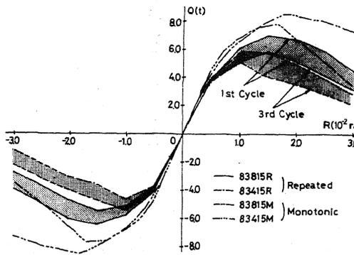
Fig. 8 Effect of Cyclic Loading
