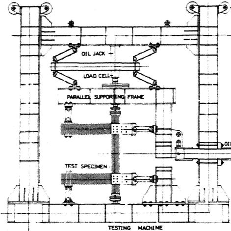
Fig. 3 Loading Apparatus
