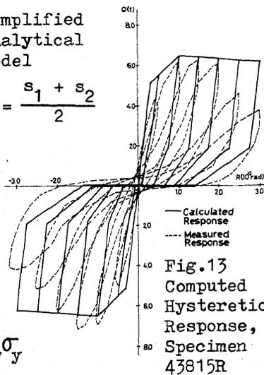
Fig. 13 Computed Hysteretic Response, Specimen 43815R
