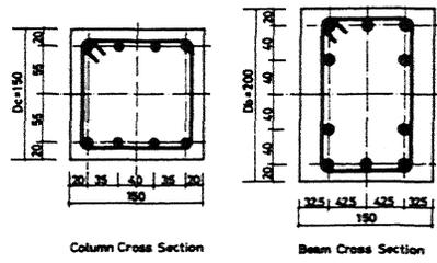
Fig. 1 Details of Cross Section
