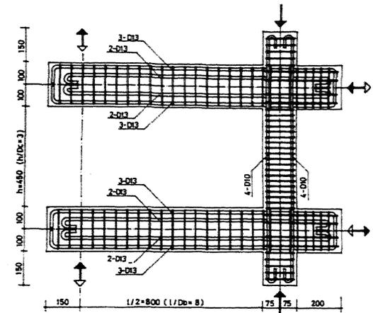
Fig. 2 Dimensions and Arrangement of Reinforcements, Specimen 83830R
