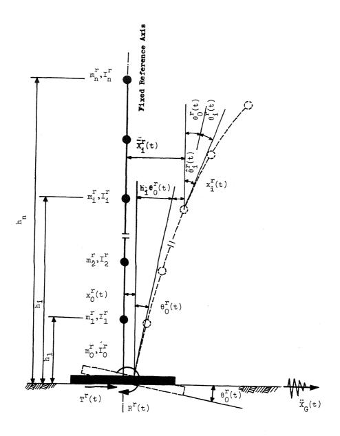
Fig. 1 - Structure-Foundation-Soil System
