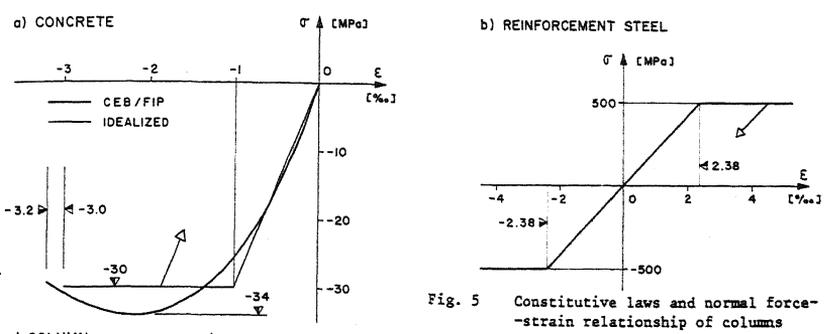
Fig. 5 Constitutive laws and normal force-strain relationship of columns
