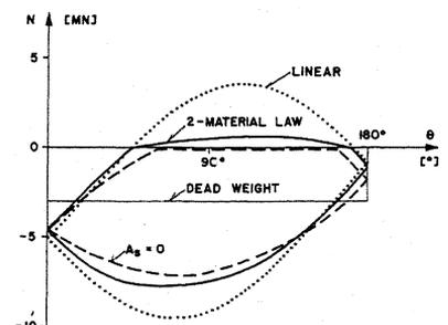
Fig. 8 Normal force in column versus circumferential angle,  $t = 2.7$  s, DBE (0.12 g)
