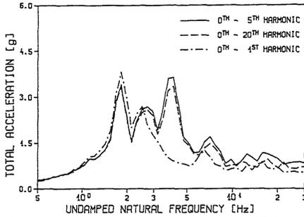
Fig. 10 In-structure response spectra (1% damping), x-direction, top of shell,  $\theta = 0^\circ$ , 2 material law, 2-DBE (0.24 g)
