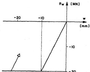
Fig. 6 Vertical reaction-displacement relationship of separate foundation
