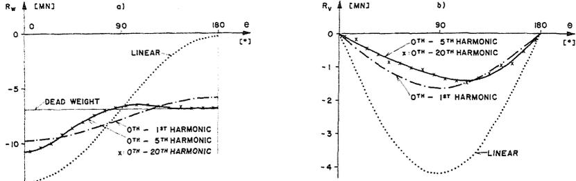
Fig. 11 Reaction force versus circumferential angle,  $t = 2.7$  s, 2-material law, 2-DBE (0.24 g)
