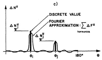
Fig. 7 Mathematical procedure to incorporate nonlinearity of column
