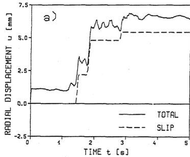
Fig. 12 Horizontal displacement of separate foundation at  $\theta = 105^\circ$  versus time, 2-material law, 3-DBE (0.36 g)
