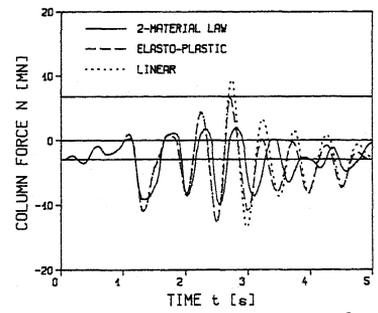
Fig. 9 Normal force in column at  $\theta = 105^\circ$ ,  $a < 0$  versus time, 2-DBE (0.24 g)
