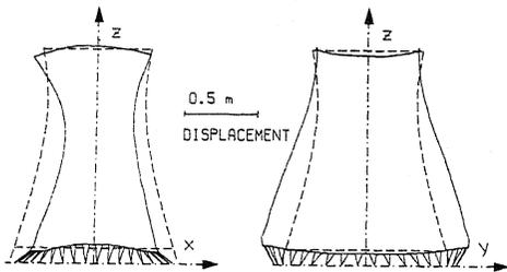
Fig. 14 Permanent displacement after earthquake, 2-material law, 5-DBE (0.60 g)
