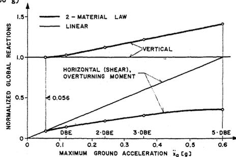
Fig. 15 Maximum global reactions versus level of earthquake excitation, 2-material law
