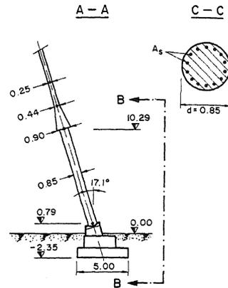
Fig. 2 Geometry of supporting columns
