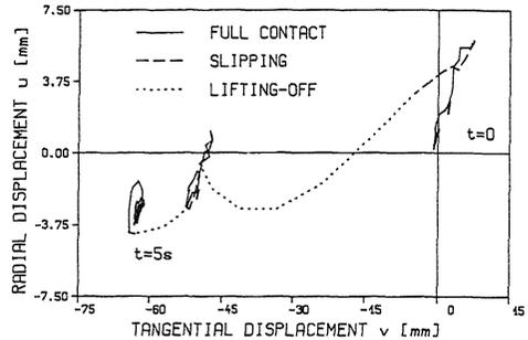
Fig. 13 Horizontal displacement of separate foundation at  $\theta = 145^\circ$  versus time, 2-material law, 5-DBE (0.60 g)
