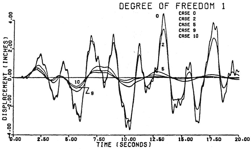
Fig. 4 Structure Response to the 10.4 second Ft. Tejon Record for Different Cases of Damping
