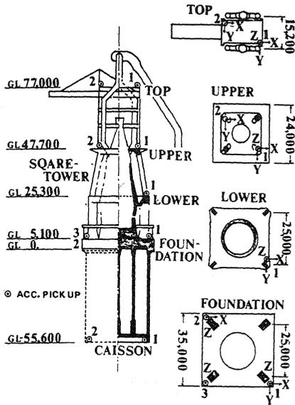
Fig.1 Outline of No.1 blast furnace
