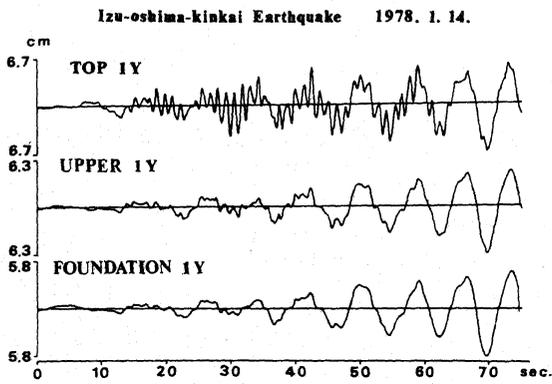
Fig.4 Observed displacement response waves
