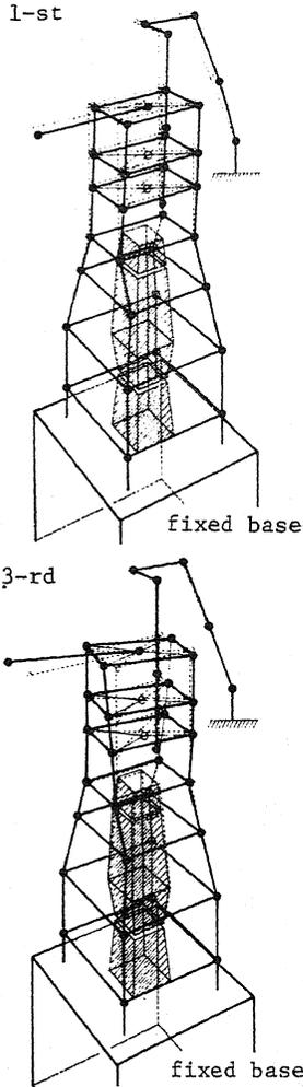
Fig.6 Normal modes of No.1 blast furnace
