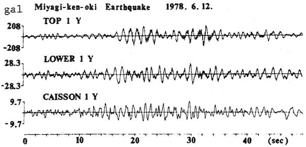
Fig.5 Observed acceleration response waves
