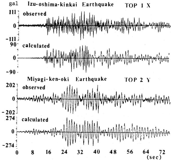
Fig.7 Comparison of observed and calculated acceleration waves
