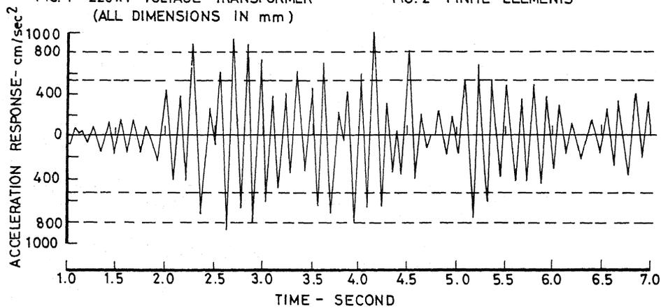
FIG. 3 - TIMEWISE ACCELERATION RESPONSE OF V. T.
