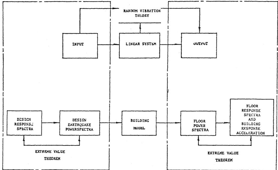
FIGURE 1. SCHEMATIC REPRESENTATION OF UNIFIED APPROACH FOR DETERMINING RESPONSE ACCELERATION AND FLOOR RESPONSE SPECTRA
