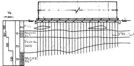
Fig. 1 Profiles of Soil and Tank.
