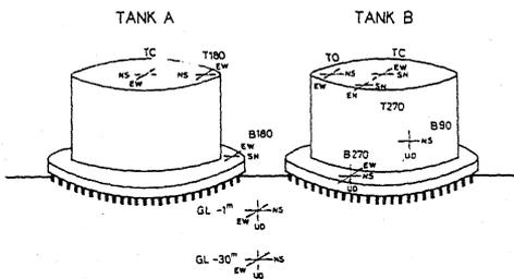
Fig. 2 Display of Accelerometers
