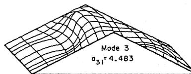
Fig 3. Modal shapes for dam in rectangular canyon,  $B/H=1.5$ ,  $L/H=3$ ,  $j=1$
