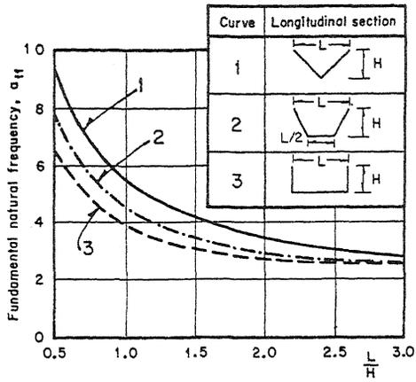
Fig 4. Fundamental natural frequency for dams of various longitudinal cross-sections; B/H = 1.5
