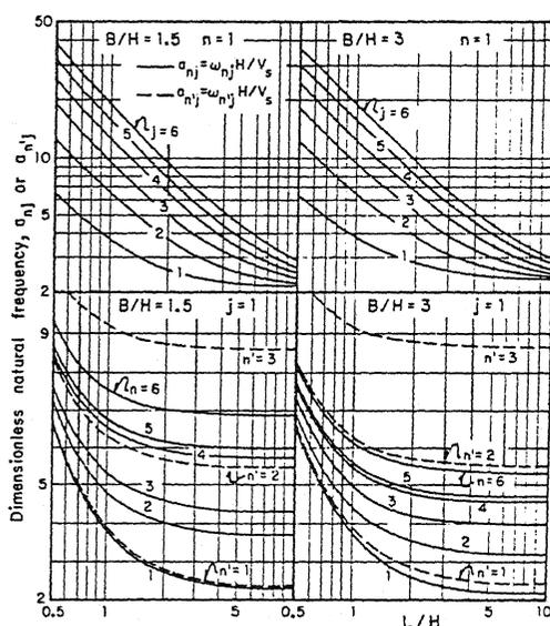
Fig 2. Natural frequencies for homogeneous dam in rectangular canyon
