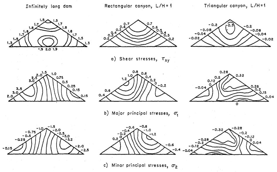
Fig 6. Stress contours in  $\text{kg/cm}^2$  for midplane for a given instant of time,  $t = 2.26$  sec; B/H = 1.5
