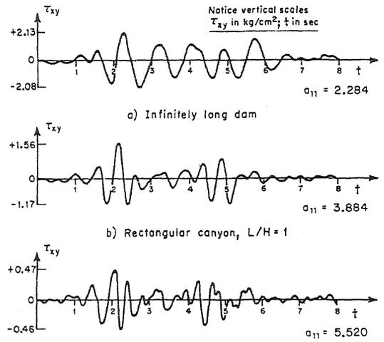
Fig 5. Time history of shear stress at a point on vertical axis of symmetry, 30.5 m high; B/H = 1.5
